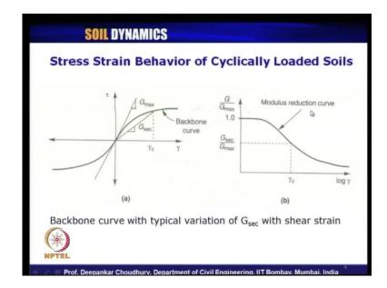
And from that we have seen what is called backbone curve, the plot of tau versus gamma is known as backbone curve. And if we represent it in a non dimensional form of G by G max versus the log scale of the cyclic shear strain and if we plot any data. The typical
