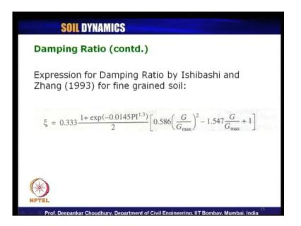
And the expression to compute the damping ratio value is proposed by Ishibashi and Zhang in 1993 for fine grained soil they again used mostly the soil from the Japan region. So, this is the symbol for damping ratio they have been used is given by this expression it is depended on the value of G by G max and the plasticity index. So, that is why when you are taking the G by G max at which particular value of cyclic shear strain you are using that automatically is taken care that effect.
