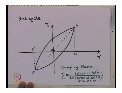
Third cycle of the hysteresis curve is called a representative cycle to compute the value of damping ratio. So now, let me plot the hysteresis curve for a typical third cycle let us say the hysteresis curve looks like this, this is for third cycle am using. So, let me give the nomenclature of various points, because it will require for us to compute the damping ratio of the system; let us say this is the origin, this point is say A, this is B, this is A dash this one is B dash.
