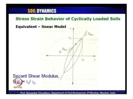
So, coming to the slides the stress strain behavior for any cyclically loaded soil, this is the equivalent linear model with G secant modulus.
