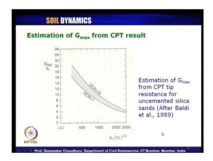
Now, some more estimation of G max value from cone penetration test result, as was proposed by Baldi et al in 1989, that they have used not only normally consolidated soil
