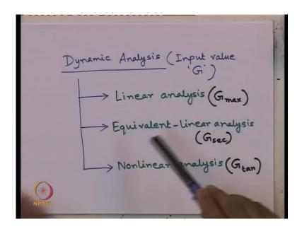
We can sub classify the any dynamic analysis into three categories linear analysis, equivalent linear analysis and non-linear analysis; based on what is our input value of the shear modulus we are using for the analysis. When we are using the maximum shear modulus it is linear analysis, which we have seen that it is the most easiest or simplest analysis, because he had the value of g max remains constant throughout the analysis.
