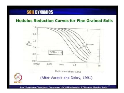
So, let us look at modulus reduction curve for fine grained soil, this is also proposed by Vucetic and Dobry in 1991. Modulus reduction curve means we know g by g max in the y axis and x axis is log scale of the cyclic shear strain which is applied to the sample. So, this the lab test result; obviously, as we know the curve should start at this G by G max at one at very low strain level and then with increase in strain they will keep on decreasing.
