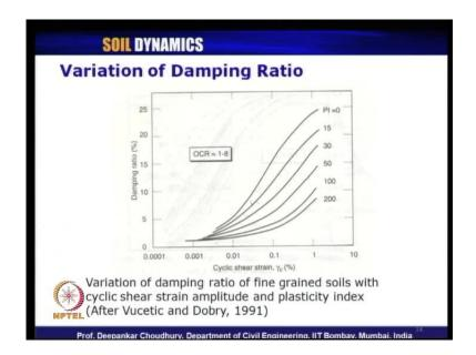
Now, coming to the next important parameter dynamic soil property is damping ratio. So, the most important dynamic soil properties are a g value shear modulus and damping ratio. Now, coming to the damping ratio how to estimate the value of damping ratio.
