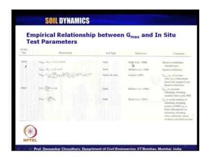
Other relationship have been proposed by several other researchers also depending on in situ test parameters that is standard penetration test value or cone penetration test value to compute the G max. Also the dilatometer test value or pressure meter test value also the G max can be computed as was proposed by several other researchers for different types of soil.
