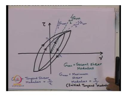
First let us look at this page that is any cyclic test in the laboratory, we can get the data for cyclic shear test versus shear strain. So, the plot of shear test versus shear strain we will start from this point origin 0, 0; it will go up in the loading curve, then if we release the load because this is a cyclic load, this is unloading curve and then again reloading curve. So, like that these are the cycles as per different cycles, we will get different envelope of this tau versus gamma plot.
