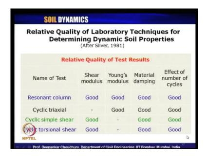
Now, let us come to the relative qualitative assessment for various laboratory test, what we have seen to determine the dynamic soil properties. It is given by silver in 1981 this column gives the various names of the laboratory test, that is resonant column test, cyclic triaxial test, cyclic simple shear test, cyclic torsional shear test. And these are the parameters which we are obtaining shear modulus, young's modulus, material damping and effect of number of cycles.
