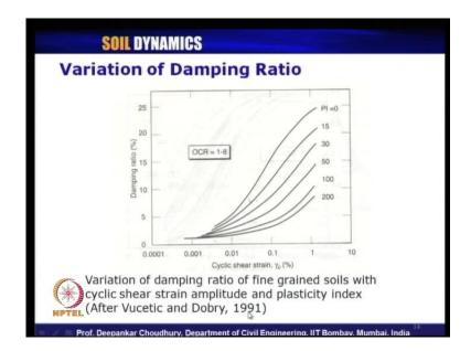
So, again the work of Vucetic and Dobry in 1991 for fine grained soil as been reported here for different values of cyclic shear strain how the damping ratio behaves it is represented in percent. And for various soil they have considered OCR value between 1 to 8 and for different value for plasticity index they have plotted the curve.
