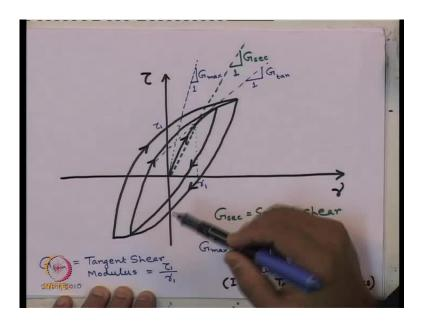
Let us look at this picture once again from any cyclic load test we are getting a typical curve like this, which is known as hysteresis curve, this tau versus gamma plot for different number of cycles of loading. Now, among these curves the third cycle is called the representative cycle.
