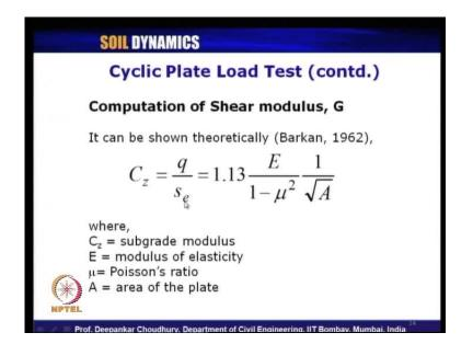
Now, how to compute the shear modulus from the cyclic plate load test it can be shown theoretically as proposed by Barkan in 1962 that C z, C z is defined as sub grade modulus similar to our static case of soil sub grade modulus. What is sub grade modulus the unit of sub grade modulus is nothing but pressure per unit displacement right. So, in this case from the cyclic plate load test the sub grade modulus, dynamic sub grade
