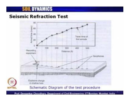
Also for seismic refraction test.
