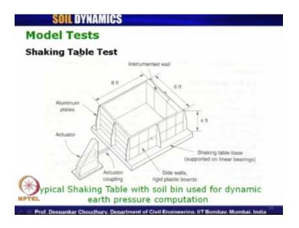
Within model test, we have seen what are the basic fundamentals about the shaking table test and what are its direction of shaking; depending on that we can have one-directional, twodirectional or bidirectional or multidirectional shaking table facility testing facility. (Refer Slide Time: 04:11)
