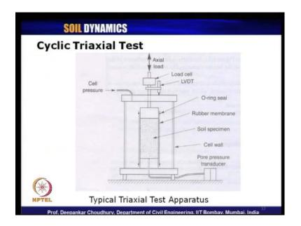
Again for the cyclic triaxial test, we have seen what is the basic methodology or basic difference between the conventional triaxial test with the cyclic triaxial test; only we use this deviatric load as cyclic in nature. And also in this test we have seen, we can do not only the isotropic C D and CU test, but also an isotropic test.
