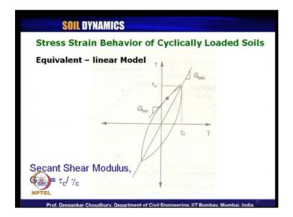
Now coming to today's lecture, let us first discuss about when we conduct in laboratory, suppose the second category of test; that is the sample test with high strain level. So, suppose we are conducting in laboratory the cyclic triaxial test or cyclic simple shear test, what finally we can get the result or what we can draw, let us draw here.
