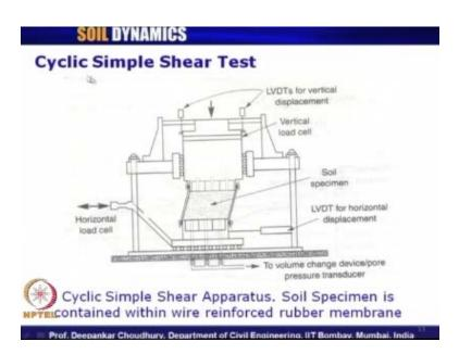
Then, we have seen what is the basic concept of cyclic simple shear test in direct shear apparatus when we apply the shearing load in the horizontal direction instead of static load; we apply in the case of cyclic simple shear test, the dynamic load or cyclic load.
