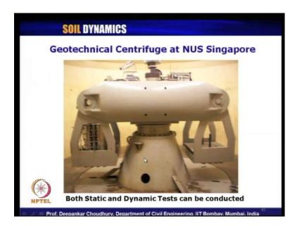
Some of the world class centrifuge testing facilities where dynamic test can be done; only a very very few and limited organizations can do the dynamic centrifuge test, some of them I am listing here for your knowledge. At National University of Singapore, this is their drum type centrifuge, this is counterweight part, and this is the bucket where the soil sample with container wheels placed. So, here they can do the dynamic test and as well as the static test.
