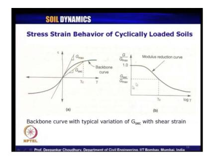
Now another terminology is used for this curve of tau versus gamma for any soil sample when it is cyclically loaded; that curvature that curve of tau versus gamma is called backbone curve. So, what is backbone curve refers to in a dynamic soil properties problem related to? It is nothing but the output of shear stress versus shear strain plot of any cyclically loaded soil; the curvature that curve is called backbone curve.
