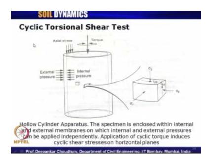
Also we have seen the cyclic torsional shear test.
