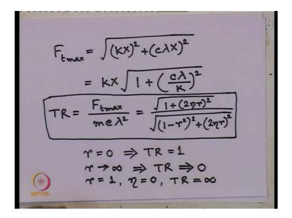
So, F t max is given by root over K X whole square plus C lambda X whole square, which we can simplify like this K X we can take out, 1 plus c lambda by K whole square,
