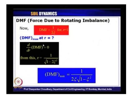
Also we have computed what is the maximum dynamic magnification factor, and at which value of that frequency ratio it occurs. We obtain that the value of frequency ratio where it becomes maximum is 1 by root over 1 minus 2 eta square, where eta is the damping ratio of the system. And the value of that maximum dynamic magnification factor is 1 by 2 eta root over 1 minus eta square.
