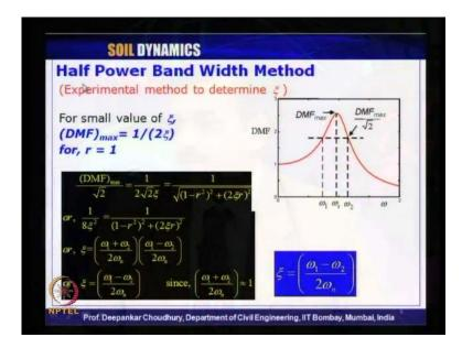
Also we have seen the concept of what is known as half power band width method, it is an experiential method to determine the damping ratio of a system. And using this concept we can find out the damping ratio, based on the applied external frequency and the natural frequency of the system expressed in this way.
