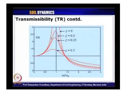
So, let us look at the plot on this slide once again, you can see it starts form transmissibility ratio equals to 1, when frequency ratio is 0 irrespective of the value of the damping ratio. And it attains it maximum for undamped case it goes to infinity at r equals to 1, and for damped system it attains a peek little before r equals to 1 that is r little less than 1, the maximum is obtained. Here also you can easily find out, what is the
