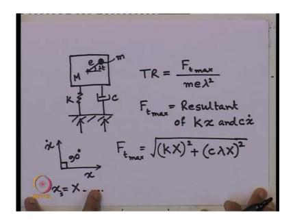
So, let me draw a single degree of freedom system here, with a rotating imbalance, so I am considering a system which is having a rotating mass of small m, and this is lambda t, e is the eccentricity and capital M is the mass of the total system, this is stiffness k, this is damping c. So, the transmissibility ratio TR, it is expressed as the maximum value of force transmitted divided by the amplitude of the force applied to the system.
