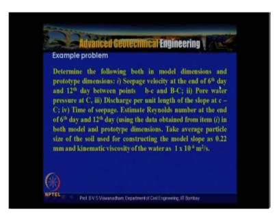
And what we need to do is that seepage velocity at the end of the 60-day and 12 today between points bc and bc that will be shown and pour water pressures and discharge per unit length of the slope at the C&C and time of seepage so average particle size is given as point 22 mm and kinematic viscosity the water is given as 1 cent a stroke that is 1 into  $10^{-6}$  meter square per second.
