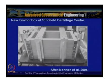
So this is a typical laminar box at the schofield centrifuge Center wherein you can see that you have what different types of aluminum discs which are actually placed and contained in this direction as well as the, so for shaking in this direction and also they contained in this direction so this is you know said the distance is said depending upon the whatever the amplitude is allowed, so this is atypical model container in National University of Singapore.
