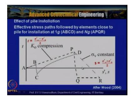
So here on the x-axis the S which is  $\sigma v' + \sigma h' / 2$  is plotted sand t which is nothing but  $\sigma v' - \sigma h' / 2$  is plotted. So and here is actually shown and this is the k0 compression line and effective stress parts followed by elements close to the pile for installation at 1g we are in that it follows that a b c and d.
