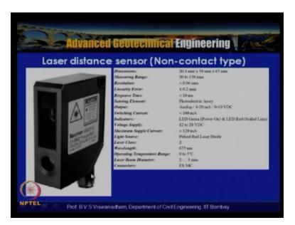
Non-contact type and so this is what actually is being shown at the through this actually the light is actually shown then this is a connected to the data acquisition system.
