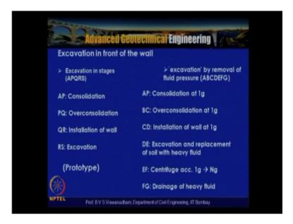
By removal of fluid pressure ABCD EFG so AP which is actually consolidation and PQ is war consolidation that is the removal of the load and QR installation of wall and RS is the excavation so if you look into this AP is consolidation that is along the compression line and then we have seen that PQ war consolidation so PQ is or consolidation release and a QR is what we said is that installation that is the driving of the wall and RS is the excavation that is the RS is the excavation.
