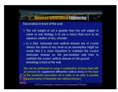
So the unit weight of the soil is actually greater than the unit weight of water so this strategy is to use a heavy fluid such a ways that aqueous solution of zinc chloride can be used so in a fluid if the horizontal and vertical stresses are of course always same in any level so an assumption might be made is more important to maintain the correct horizontal stresses on the preinstalled wall then to maintain the correct vertical stresses on the ground remaining in front of the wall.
