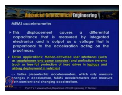
So the displacement causes a differential capacitance that is measured by the integrated electronics and is output as voltage that is proportional to acceleration acting on the proof mass so you know this is you know the basic you know principal and the applications earlier applications include motion activated user interface such as in smart phones and enter game consoles and protection systems such as free fall production of hard drives in laptops and airbag deployment in vehicles.
