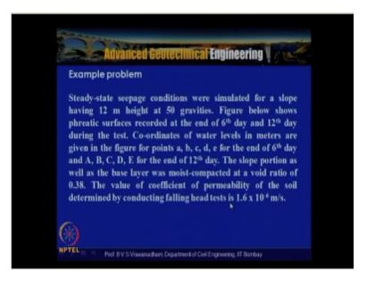
So this particular example problem basically consists of steady-state problem conditions were simulated for aslope having 12 meter height at 50 gravities and figure below shows us the shows the you know pre attic surface are given and these are actually obtained from this interface model test and the slope portion as well as the base layer was moist compacted in void ratio 0.38 and the question the perimeter the soil is  $1.6.10^{-6}$  meter per second.
