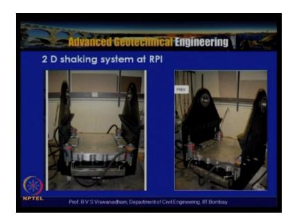
So this is the typical two-dimensional shaking system available at RPI and you art and wherein you can see that the swing basket package will come out of the chamber along with the earthquake actuator that means the earthquake actuator fitted in a soul basket and they use this for performing earthquake experiments and for the rest of the experiments they will use a different basket, so this particular slide shows the use of a you know earthquake actuator mounted on the swing basket.
