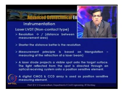
And the resolution is the function of distance between the transducer and measure measurement area and the shorter the distance better the resolution and the measurement principle is based on the triangulation and the measuring of the refraction of a large supreme, so what will happen is that you have a you know this razor transducer and which actually throws a you know a light on the subject or object, so what will happen is that the refraction is actually received in a same transition.
