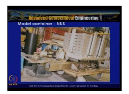
Small one dimensional shaking system and wherein we have the earthquake actuator.
