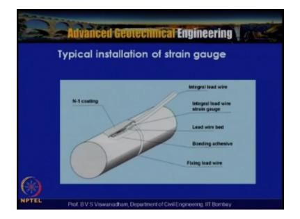
So this is the typical installation of a strain gauge on a pile and for some convenience to avoid some roughness one can actually also take the leads through the pipe is actually hollow can be taken through the through the pipe. (Refer Slide Time: 22:47)
