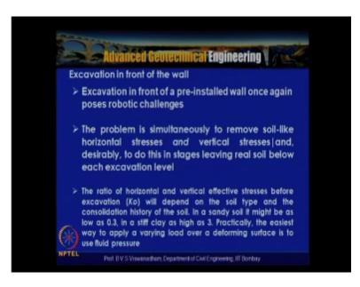
So for the excavation in front of the wall basically you for a preinstalled wall once again this actually poses robotic challenges and the problem is some it you know the simultaneous removal of soil like horizontal stresses and vertical stresses and desirably to do this in stages leaving real soil below each excavation level that is actually the requirement.
