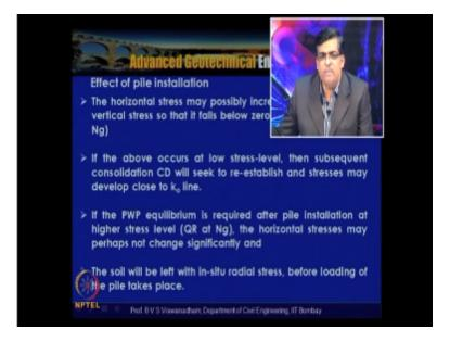
So let us explain this the horizontal stress may possibly increase even above the vertical stress so that it falls below zero bc at NG+ PQ at NQ that is that this horizontal stress increases because of the pile ride so it falls below zero and bc incase of 1NG installation and then PQ in case of NG installation if the above you know the variation occurs at low stress level then subsequent consolidation CD will seek to reestablish.
