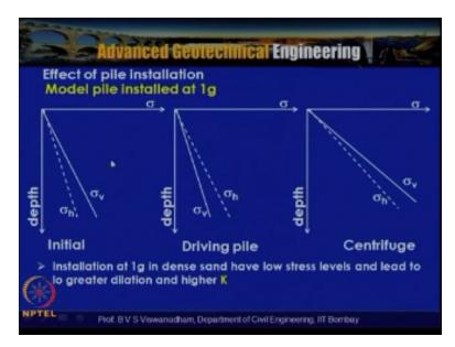
And the  $\sigma$  mean  $\sigma$  H or the you know if you take an element very close to the pile then  $\sigma$  V is the vertical stress and  $\sigma$  H is ours and stress, so because of the low stresses the stresses are low there
