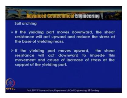
If the yielding part moves downward that means that the soil above the conduit the shear resistance will act upward and reduce the stress at the based on the yielding mass so what will happen is that if the yielding part moves downward means that the soil above the conduit the shear resistance will act upward and reduce the stress at the based on the yielding mass.
