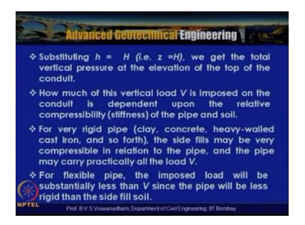
So when you seen is that in the previous equation when  $v=\gamma cd*bd2$  where by substituting for cd expression when h=h or z=h we get the total vertical pressure t the elevation of the top of the conduit now how much of this vertical v load we imposed on the conduit is dependent on the pipe and soil.
