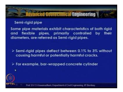
So we have seem that flexible pipe nd rigid pipe in the flexible pipe were in the soil above the pipe will undergo settlement and o because of this the shear resistance participation of active arching and or we can say favorable arching there is the reduction of the load coming on to the pipe so the buried conduits will experience the less load so there is also rigid pipes and then we also said that there is one more category called semi-rigid pipes.
