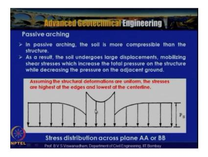
So in case of passive arching the soil is more compressible than the structure so passive arching occurs when the soil is actually more compressible than the structure so as a result the soil undergoes large displacements at mobilization of shear stresses which increase the total pressure on the structure while decreasing the pressure on the adjacent ground.
