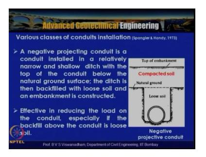
There is also another class of projecting conduits is called a negative projecting conduits a negative projecting conduits is called is conduit installed in a well thoroughly narrow and a shallow ditch with top of the conduit below the natural ground surface and the ditch is then backfilled with loose soil and an embankment is constructed so this is you know negative projecting conduit is literally is installed in a shallow trench.
