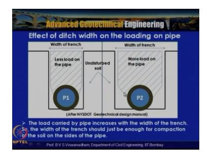
So effective of the ditch width on the loading on the pipe so here the width of the trench and the width of the suppose if you vary shaving you know less width of the trench then the pipe actually attracts less load because of the participation of the trench and if width of the trench is actually more than the load carrying the pipe increases the width of the trench.
