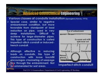
There is also other class of you know in category of conduits which is called imperfect ditch conduit this is a special case similar to negative embankment condition but more favorable from stand point of load reduction on pipe used in very deep installations and difficult to achieve for large diameter pipes and this type of construct is called imperfect-ditch conduit or the induced trench conduits.
