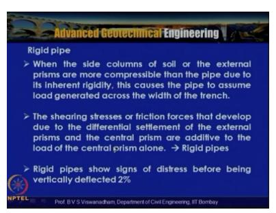
So after having seen active arching and passive arching we said that the active arching occurs when structure is you know under more flexible, more structure is in case of passive arching the soil is more compressible than the structure in case of active arching soil is you know structure is more compressible than the surrounding soil okay.
