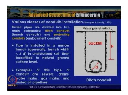
That is which are required nowadays to be embedded below the crowd level and these are off shore as well as on shore so this buried pipelines are divided into two main categories and these are called as ditch conduits that is conduits which are embedded in ditch or in trench and as not all conduits can be put blow the long level so that a some of the conduits will representing out above the ground surface their called embankment conduits or projecting conduits.
