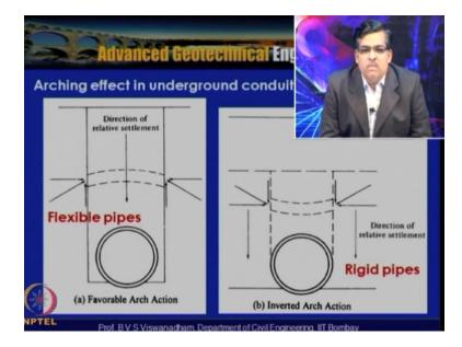
Now here the typical favorable art conditions are actually shown arching effect is underground conduits you can see that here this is a flexible pipes so where the direction of the relative settlement will be here in this direction the resistance from this side walls actually act upwards so because of this load acting in the central position will be less so in this case you know arch action.
