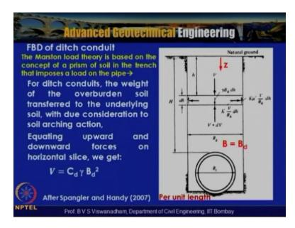
So in this particular slide you are free boding slide diagram of the ditch conduits which is actually shown here a type of the diameter external diameter BC and are conduit of BC and internal diameter let us say a small d and width of the trench is indicated here as BD but for the terminology we can also write BC=BD and so net Z is the depth form the natural ground
