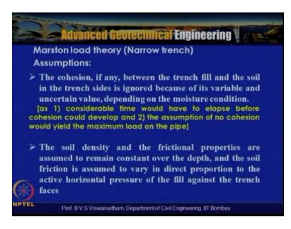
So in going to understand about Marston load theory for narrow trenches and let us look into the assumptions which are put forwarded here the cohesion if any between the trench fill and the soil in the trench side is ignored so the primary the cohesion if any between the trench fill and the soil in the trench sides is ignored because of its variable and uncertain value depending upon the moisture condition.
