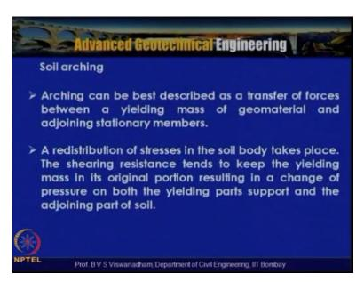
So now let us try to understand about the soil arching, soil arching can be you know the best described as the transfer of the forces between yielding mass of geo material and adjoining stationery members so arching can be best described as a transfer of forces between yielding mass of geo material and adjoining stationery members.
