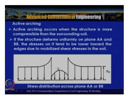
Then at plane AA or BB a stresses on its tends to be on the lower towards the edges due to the mobilized shear stresses in the soil so because of the mobilized shear stresses the stress will be lower and then you can see that surrounding reads that is the non yielding portions or actually receiving the higher stresses so this is you know terminology of you know defined as the active arching, active arching occurs when the structure is more compressible than the surrounding soil.
