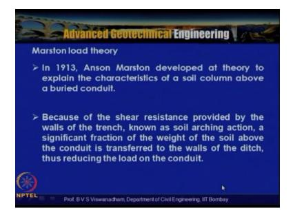
So we have seen different types of you know the conduits installations nd accordingly Marston as actually proposed in a load theory in 1913 so in 1913 Anson Marston developed at theory to explain the characteristics of soil column above the buried conduit so because of the shear resistance provided by the walls of the trench known as the soil arching so we need to understand what is this soil arching, soil arching is a phenomenon in which transfers the forces or stresses to the zones.
