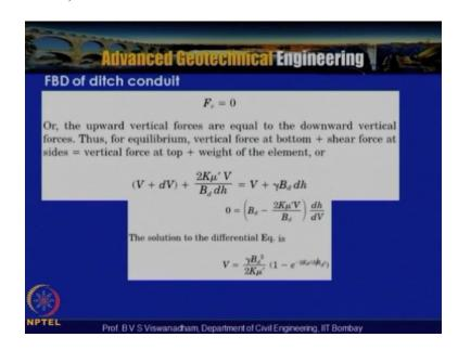
So this is what actually described here for  $\sigma fv=0$  taking upward vertical forces or equal to the downward vertical forces so for equilibrium vertical force at the bottom plus shear force at the sides is equal to vertical force at the top plus weight of the element on the slice so vertical force at the bottom that is the bottom of the slice and shear force at the sides is equal to vertical force at the top and weight of the element.
