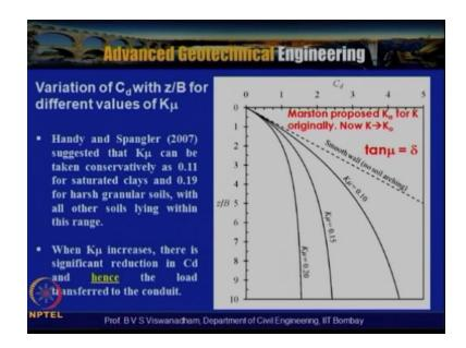
Now let us look variation of cd with z/b for different values of K $\mu$  so what we said is that this particular graph which is actually shown were cd is plotted on the x axis from 0 to 5 that is the load cohesion so z/b which is z=0 at the top of the that is the ground surface and for low arching no soil arching the smooth wall we can see that you know the this particular tends to the somewhere here.
