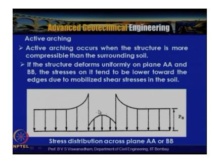
So in this case active arching occurs when the structure is more compressible than this surrounding soil so in active aching occurs when the structure is more compressible than the surrounding soil so if the structure deforms uniformly on plane AA and plane BB the stress on it tend to be lower toward the edges due to mobilized shear stresses in the soil.
