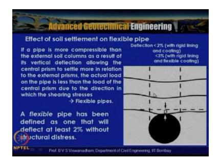
Now consider the flexible pipe if the pipe is more compressible than external soil columns as a result of vertical deflections allowing the central prisms to settle more in relation to external prisms then the actual load on the pipe is less than the load of the central prisms due to the direction in which the shearing stress are acting.
