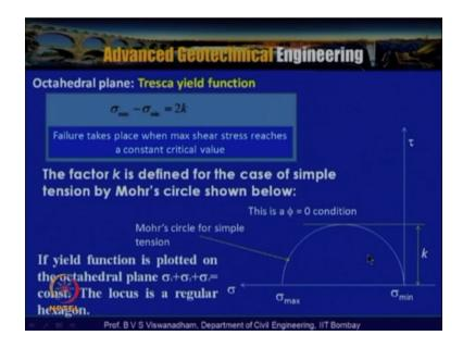
Now the octahedral plane is also given on stress presented by tresca on the tresca yield function so which is nothing but the tresca criterion or tresca function is defined as  $\sigma$ max- $\sigma$ min=2k,  $\sigma$ max- $\sigma$ min=2k, where factor k is defined by the case of a simple tension by Mohr circle actually shown in the slide. So this indicates that failure takes place when the difference that is max shear stress reaches a constant critical value.
