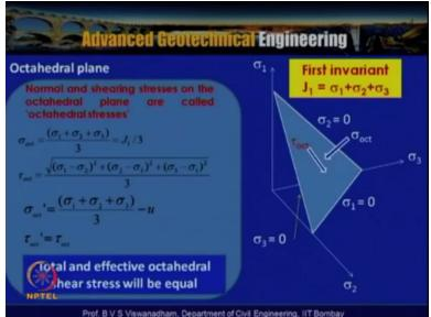
So we have you know this octahedral you know  $\sigma$  octahedral this is the normal stress and this is the shear stress,  $\sigma$  oct and  $\sigma$  this  $\tau$  oct. So any state of stress can be represented by two components states of stress one is you know the component consisting of equal tensile stresses, tensile or compressive stresses acting in all directions and the another one is that component of shear stress consisting of 8 octahedral shearing stresses.
