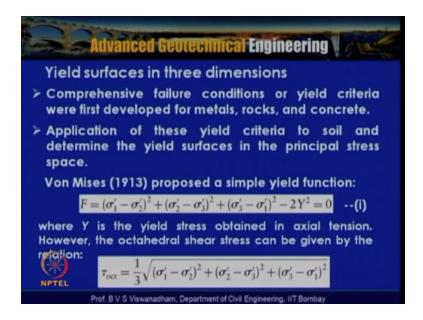
Especially the comprehensive of failure conditions or yield criteria are first developed for metals, rocks and concrete. So this comprehensive failure conditions or yield criteria basically they are developed for you know metals, rocks and concrete, now let us consider the application of this yield criteria to soil and determine the yield surfaces on the principal stress space.
