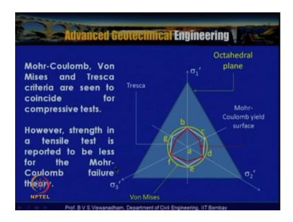
The Mohr Coulomb Von Mises and Tresca criteria are actually seen to coincide for the compressive test, so the different failure surface are actually shown here and basically here we have the octahedral plane and the tresca surface which is actually shown here and Mohr Coulomb failure surface is actually shown here and the round surface that is actually this is the tresca and this is the Von Mises failure surface which is actually cylinder circular cylinder this is the circular cylinder.
