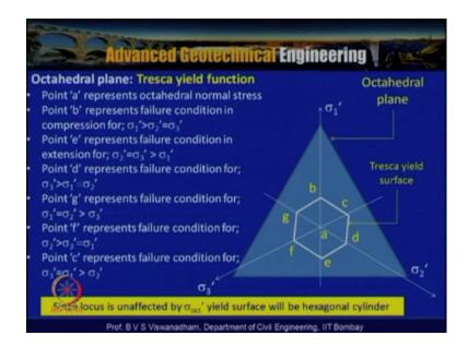
So the tresca yield surface on the octahedral plane is actually represented where bcdefg these shown here which is where similar to Mohr Coulomb failure surface, but a is the you know the point through which the hydrostatic axis or you know where  $\sigma 1 = \sigma 2 = \sigma 3$  is ensured and where bcdef and g so a represents the octahedral normal stress the point passing through the octahedral normal stress passes and b represents the failure condition in compression.
