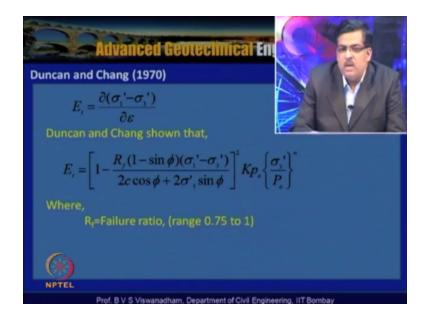
And according to Duncan and Chang 1970 where Et that is nothing but  $\partial(\sigma 1 - \sigma 3) \partial \epsilon$ , so Duncan actually have shown that the E value that is Et=[1-Rf(1-sin $\phi$ )( $\sigma 1' - \sigma 3'$ )/2c cos $\phi$ +2 $\sigma 3'$ sin $\phi$ ]<sup>2</sup> Kpa9 $\sigma 3$ /Pa)<sup>n</sup>.
