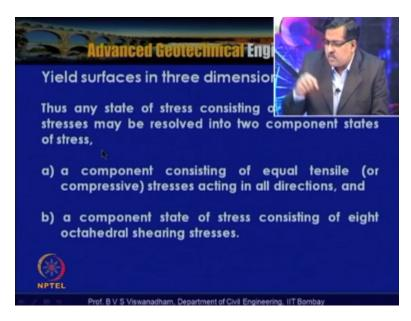
And further the any state of stress consisting of three principal stresses like  $\sigma 1 \sigma 2 \sigma 3$  may be resulted into two component states of stress and these are called octahedral stresses one is octahedral normal stress octahedral shear stress. A component consisting of equal tensile stresses you know acting on in all directions and a component state of stress consisting of 8 octahedral shear stresses. (Pafer Slide Time: 10:44)
