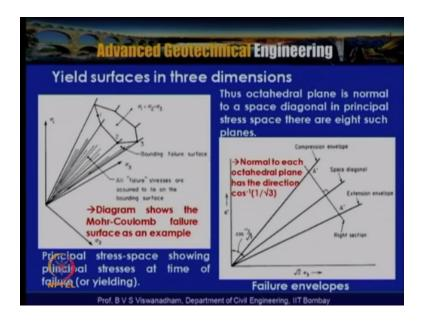
Now here the yield surface in three dimension is shown here so here with  $\sigma 1 \sigma 2 \sigma 3$  and for example here the diagram shows the Mohr Coulomb failure surface as an you know hexagonal shape here and this is the bounded failure surface and here all failure stresses are assumed to be in the bounding surface so all failure surface, failure stresses are assumed to be on the, they are assumed to be on this boundary surface.
