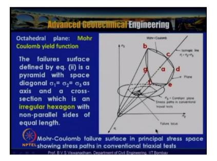
Now the failure surface is defined by equation 2 that is basically this one is a parameter, basically is a pyramid with space diagonal which is  $\sigma 1 = \sigma 2 = \sigma 3$  as axis that is the isotropic line or hydrostatic axis which is actually called as  $\sigma 1 = \sigma 2 = \sigma 3$  as axis and a cross section which is an irregular hexagon with non parallel sides of equal length.
