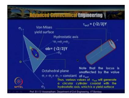
And this is represented further in depth here as this is the octahedral plane and this is the Von Mises yield surface and ab is nothing but  $\sqrt{2}/3$ Y and this is the hydrostatic axis  $\sigma 1 = \sigma 2 = \sigma 3$  and so this Von Mises failure surface is you know you can see like a circular cylinder having with coaxial with you know hydrostatic axis this cylinder is actually the diameter is the radius is equivalent to ab here, where ab= $\tau oct = \sqrt{2}/3$ Y.
