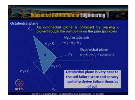
So this is the octahedral plane which is actually shown you know the octahedral plane is obtained by passing a plane through the unit points on the principal axis, so in this particular slide what we see is that  $\sigma 1$  and  $\sigma 2$  and  $\sigma 3$  and this is the hydrostatic axis where  $\sigma 1 = \sigma 2 = \sigma 3$  so this is the hydrostatic axis and the line joining this points which are actually this particular plane is called as octahedral plane.
