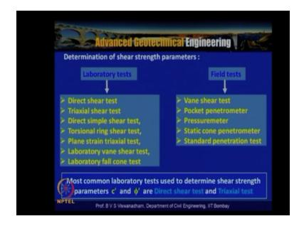
So the different determination of the shear strength parameters can be achieved through laboratory or to field this and the laboratory predominantly the direct shear test and trashy tests are performed you know traditionally and there are also some other classes of tests like direct simple shear test and tensional ring shear test, and plane strain to axial test and for very soft soils we wanted to determine whether the sample making is difficult that in that case.
