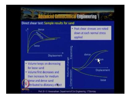
So in this particular figure the typical you know shear stress versus shear displacement for loose sand and mediums and dense and actual are given so as can be seen that you know loose and actually has got you know the continuously the hardening effect can be seen but in case of a you know the medium sand and then sand and particularly for dense and there is a predominantly a peak is actually observed and then once the peak stress is actually.
