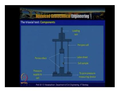
So this is the you know typical component of a tri-axial test where you actually have what a sample and a chamber in which you know what you have is that you know the confinement is actually provided in the form of filling the water so initially when the sample is actually place
