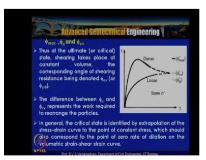
So let us try to you know interpret between  $\pi$  max and  $\pi \mu$  and a  $\pi \operatorname{cv} \pi \operatorname{CV}$  is the friction A angle at a constant volume and CV indicates at you know at constant volume and so in this particular slide at  $\tau$  axis you know shear strain is actually shown here and where for dense sand and loose and the shear stress variations are shown here as can be seen that the shear stress is actually maximum here.
