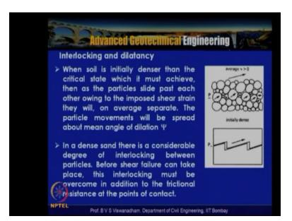
So let us look into this interlocking and you know dilatancy phenomenon's when soil is actually is initially denser than the critical state where critical state is the place where no volume change occurs which it must achieve then as particle slide past each other going to the imposed a shear strain in our way they are an average they actually tend to get a separate and the particle movements will be spread about a mean angle of dilation that miscalled sign and in a dense.
