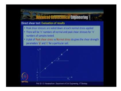
But let us look into the interpretation of the direction your test results and then you know we will try to look into some example and here the peaks shear stresses are noted from the shear stress versus shear displacement or shear strain curve and each normal stress the peak stress is actually when it is picked up and when it is plotted here and the line joining this you know this elope is actually resulted as a Mohr- Coulomb failure elope.
