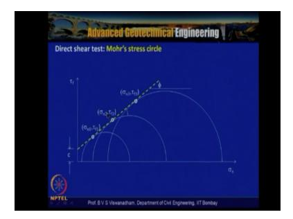
And further you know there is a way very we can actually construct the more circles because here in this case what we are trying to do is that we can actually construct the Mohr-coulomb failure runner up and we know actually this particular point so what we can do is that you know the this point you know more circle more Mohr- Coulomb hypothesis actually states that when more subtle is in contact with the failure analog.
