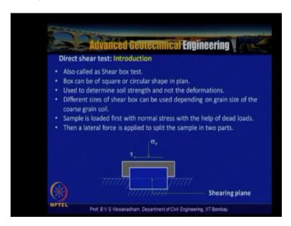
So let us look into the first the direct shear test and it is also called as a shear box test and this box can be square or circular in shape and this box sizes are predominantly 60 mm x 60mm or we have 100 mm /100mm or 300 mm/ 300mmso depending upon the size of the particles which are actually involved and to prevent the scale effects the sizes of the you know the direction boxes need to be adopted and is also used to determine.
