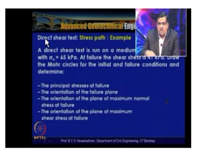
So let us consider an example where in a direct shear test is actually run on a medium dense and dense sandy silt with normal stress of 65 of Pascal's at failure the shear stress is observed as 41 kilo Pascal's and draw the more circles at the initial and failure conditions and determine principle stresses at failure and the orientation of the failure plane and the orientation of the plane of maximum normal stress at video orientation of the plane of maximum shear stress at failure.
