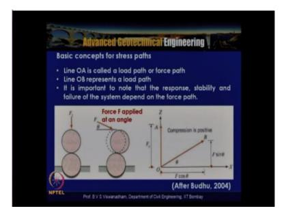
Now let us look the introduction to the stress parts in PQ space so before that let us consider, note two examples. We have on the left hand side in the figure 2 marbles or which can be represented like a 2 spherical grains which are actually you knows in figure on the left hand side here which is actually one grain is sitting on the other and assume that there is a vertical force is acting in the direction of the vertical direction.
