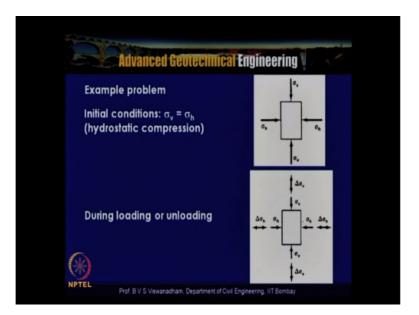
Now let us take an example problem where we have got initial condition which is hydrostatic condition  $\sigma V=\sigma H$ , you have got some cylindrical sample where you have applied vertical stress and horizontal stress, that means that the sample is confined with a hydrostatic pressure which is actually having, that means that the sample is actually with a pressurized system and then it will be subjected to  $\sigma V$  in vertical direction,  $\sigma H$  in horizontal direction.
