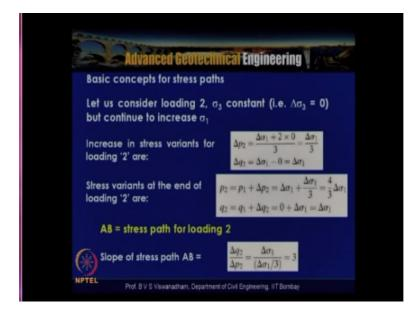
Let us consider the loading condition 2 where  $\sigma$  3 is constant that means that there is a  $\sigma$  3 which is applied, but there is no change in  $\Delta \sigma$  3. The  $\sigma$  3 is constant means rate of change of  $\Delta \sigma$  3 is constant. so  $\Delta \sigma$  3 is equal to zero which is the loading condition is indicated within two here and  $\Delta \sigma$  1 is greater than zero that means that once we held with certain  $\sigma$  3 without constant  $\sigma$  3.
