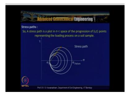
So a stress path basically is a plot which is drawn in tow  $\sigma$  space which is connecting a progression of ST where S is equal to, S and T which we have to find from the 2 dimensional point of view representing the loading process on a sample. So where you have the S = half  $\sigma$  3 by  $\sigma$  2 and T = half  $\sigma$  1 –  $\sigma$  3/2.
