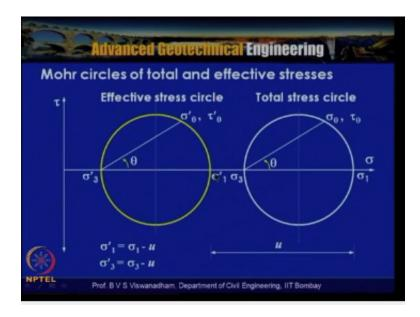
When you look at the major principle plane is here and in the effective stress conditions and minor principle plane is here, it does not change, here you can see that this is the major principle plane even in the total stress conditions and here this is the minor principal plane that is the perpendicular one in this case for the total stress condition also.
