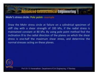
Now here with the given information two planes are possible so we could actually get for this same shear stress two different normal stresses can be seen. One is that plane inclined at 75 degrees, the other one is actually at the 15 degrees.
