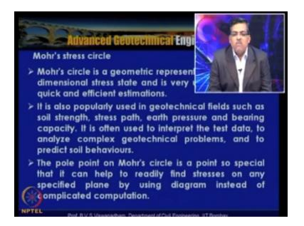
So as we have discussed, the Mohr's Circle is a geometric representation of the two dimensional stress state and is very useful to perform quick and efficient estimations, and it is also popularly used in geotechnical fields such as soil shear strength that anyhow we are going to discuss and earth pressures, varying activation of active conditions and passive conditions are discussed and also in the bearing capacity theories.
