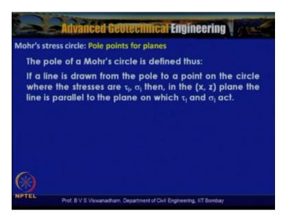
Now the pole of the Mohr's circle is defined as thus now if a line is drawn from the pole to a point on the circle where the stresses are tow i and sigma i, then in that XZ plane the line is parallel to the plane on which the tow i and sigma i act.
