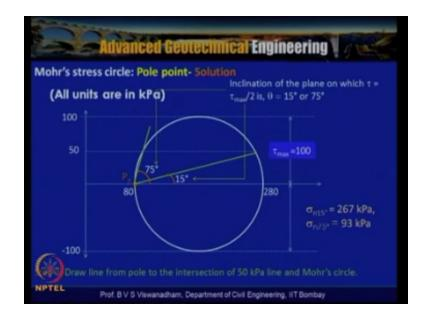
That means that when you are actually doing draw a line which is intersecting the Mohr's circle, so draw a line at tow=50 kPa which is half of tow max. Now as the principle stresses are acting on edges on the sigma 3, so here this plane is actually horizontal because the cylindrical sample, so sigma 1 is acting on the horizontal plane, sigma 3 is acting on the minor principle plane.
