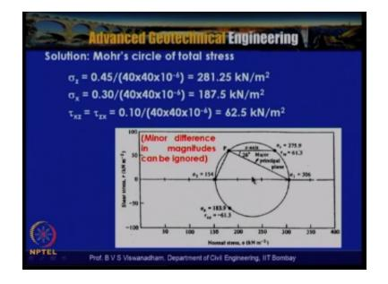
So now we do is that as we discussed we determined sigma Z which is 281 km/m2 and sigma X is 187. 5 km/m2. Now tow zx = 0.1 divided that is due to F3 and F4. So with that we have got the data, which is given based on the given data we establish sigma Z and sigma X and the tow xz and tow zx which are actually acting on the element. Now what we have done is that by knowing the stress rates here that is the magnitudes are little bit different, but however they can
