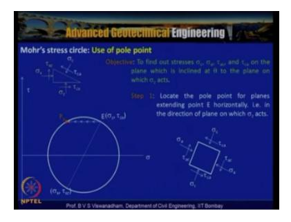
Now use of the pole point if you look into is, basically to find out the stresses sigma c, sigma a, tow ac and tow ca on the plane on which is inclined at theta, to the plane on which sigma z acts. So now we can see that, this is sigma z is actually acting on this plane and sigma x is actually acting on this vertical plane and there is tow zx is acting here and tow xz is acting here.
