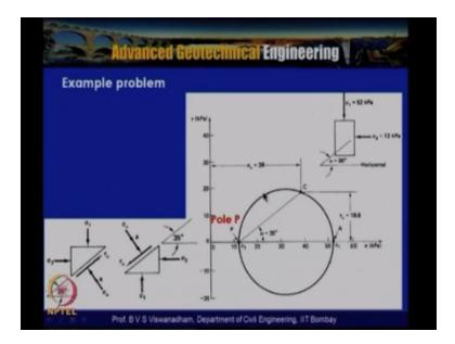
Now, another example here if you look into it, there is an element which is actually subjected to a cylindrical element, subjected to the minor principle stress is 12 kPa and major principle stress is 52 kPa. You can see that these elements are not having shear stresses so hence they can be
