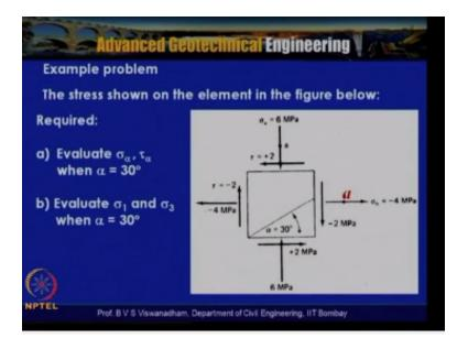
Wherein you can see that this is an element and which is subjected to, this is the horizontal plane where sigma V is equal to 6 mega Pascal's, which is actually subjected here and we have got tow is equal to 2 mega Pascal's and this is minus 2 mega Pascal's and this element is under tension and this is actually the shear stress, which is minus 2 mega Pascal's here and minus 2 mega Pascal's here.
