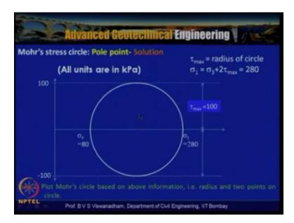
Now what has been given is that, the maximum shear strength which is nothing but 100 kPa, so that means that the maximum ordinate is actually sigma – sigma 3/2 that is tow max=100, so with this as radius sigma – sigma 3/2 as the radius, draw the Mohr's circle on tow sigma space, so then we have got the maximum shear stress with 100 kPa here minus 100 kPa here and the circle in 1, it actually intersects with sigma axis at sigma 1 it is 280 kPa and sigma 3 is 80 kPa.
