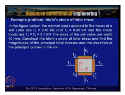
Now consider an example problem where the Mohr's circle of the total stress and element having a size of 40mm/40mm is a cube. So a two dimensional state has been actually represented here and the x axis and z axis are actually shown within the element and for estimating the shear forces and all, with muscle color filled rectangles are actually shown basically to show, you can see that this is conjugate shearing stress shear force F4, and this is the conjugate shear force F3.
