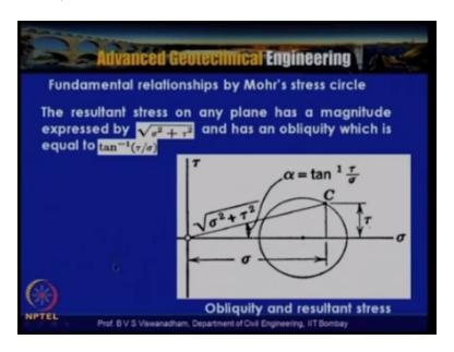
Now the other aspect is that, what is the obliquity and the resultant stress? So the resultant stress on any plane has a magnitude expressed by, we have an element, let us say sigma n tow, so the resultant is actually nothing but root over sigma<sup>2</sup> + tow<sup>2</sup> at any particular point on the Mohr's circle and has an obliquity which is equal to tan inverse of tow/sigma.
