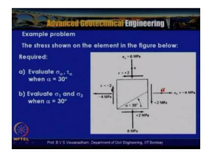
So the procedure is that plot the state of the stress on the horizontal plane that is 62 at point A and note that the shear stress makes a clockwise movement about A, so the shear stress is actually making clockwise movement about A, so from the consideration which we have defined in the previous lecture, shear stress makes a clockwise movement about A, so therefore when the shear stress is actually making clockwise movement then it is actually regarded as positive.
