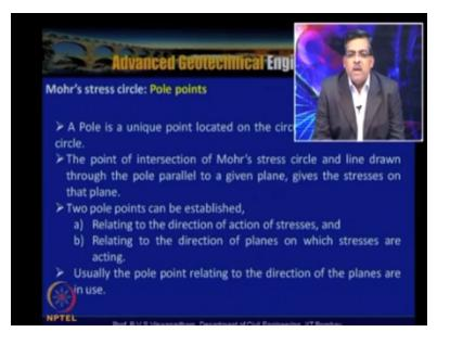
The point of intersection of Mohr's stress circle and line drawn to the pole parallel to a given plane gives the stresses on the plane. So this pole point is also called as the origin of planes. So there are two ways the pole points can be established. One is by relating it to the direction of action of stresses. The other one is the relating to the direction of the planes on which the stresses are acting. Suppose if there is a horizontal plane, if there is a normal stress acting on that.
