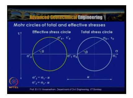
Now as we know that the total stress is nothing but effective stress plus pore water pressure. So given this condition we can actually draw a different total stresses and effective stresses. So here in this particular slide wherein we can actually see that more circle for total on effective stresses, so here on the  $\alpha$  sigma plot if you look to this on the right hand side the circle in white color indicates the total stress circle and this is nothing but the effective stress circle.
