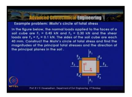
So what we have actually based on the given data, we try to establish and determine the normal stresses acting on these planes.
