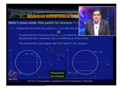
By knowing the sigma z and tow zx and sigma x and tow xz. So these are actually sigma x is normal to the vertical plane, you can see here and the sigma z is normal to the horizontal plane that is sigma z here and this is tow zx.
