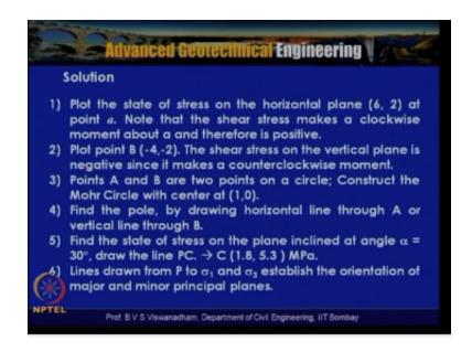
So plot the point B minus 4 minus 2, the shear stress on the vertical plane is negative since it makes counter clockwise movement, so clockwise shear stresses are positive and counter clockwise shear stresses are negative, so point A and B are two points on the circle, so construct the Mohr circle with center at 10 that is 1 mega Pascal's and zero ordinate.
