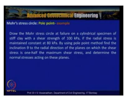
So now consider an example where you may need to draw the Mohr's stress circle at failure on a cylindrical specimen of stiff clay with a shear strength of 100 kPa, and if the radial stress is obtained constant at 80 kPa, by using the pole point method find the inclination theta to the radial direction of the planes on which the shear stress is one-half of the maximum shear stress and determine the normal stresses acting on these planes.
