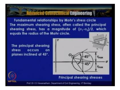
Now the fundamental relationships by the Mohr's circle can be discussed. So here tow sigma in space in Mohr's circle which is actually shown here where you can see that the stresses are actually acting sigma 1 and sigma 3 are acting on this, sigma 1 is actually acting on plane OA and sigma 3 is actually acting on plane OB and which is inclined at an angle theta. So what we need to do is that again by doing sigma 1 and sigma 3, we can draw the Mohr's circle and from
