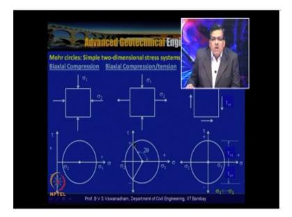
Now let us consider for some examples of the Mohr circles for different conditions of the stresses that is biaxial compression, and tension and biaxial pure shear. So here when you consider this one with  $\sigma$  1 and  $\sigma$  2 both are actually compressive stresses acting on element and two dimensional conditions have been selected and the Mohr circle represents in a towards the positive side.
