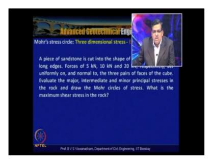
So what we have done in this particular problem is that we actually by knowing the forces subjected to the cubical shape sandstone piece, we actually have calculated what are the stresses acting on the major and intermediate and minor principle stresses and then we have drawn the Mohr circle of stress and then we also find out what is the maximum shear stress in the that rock piece.
