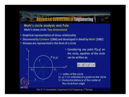
The graphical representation of stress relationship at equilibrium and discovered by Cullman in 1866 and developed in detail by Mohr in 1882. So the development actually goes back into the soil mechanics and then it is used in soil mechanics, so the stresses are represented in the form of a circle, so considering any point, P, X, Y on the circle equation of the circle can be written as  $(X-S)2 / Y^2 = R^2$  where R is the radius of the circle and X and Y are the corners of point on the circle.
