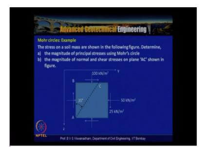
Now consider an example where the stress on a circle on a soil mass as shown in the following figure, we need to determine the principle stresses using Mohr circle and the element is actually subjected so this axis is Y axis and this axis is z axis and this plane is AB and this plane is AC. So this plane is horizontal plane and this plane is vertical plane and this is a link line plane inclined at 45 degrees to plane AB and this is the shear stresses and these are the horizontal stresses.
