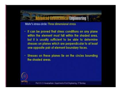
So here in this case A it can be proved that the stress conditions on any plane within the element must fall within the shaded area, that is this shaded area and it is usually sufficient to be able to determine the stresses on planes which are permanent to at least one opposite pair of element boundary faces. So in case B it is represented where you are having normal stresses and atleast two phases are actually having the shear stresses in that case we draw three Mohr circles here.
