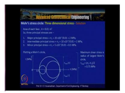
A = 0.01 meter square wherein there is nothing but 10cm x 10 cm, 100 cm2 in terms of meter it is 0.01 m2 hence three principle stresses major principle stress  $\sigma$  1 = 20 x 10 -3 /0.01, that is 2 mega Pascal's and intermediate principle stress which is nothing but  $\sigma$  2 which is 10 x 10 -3 /0.01 is one mega Pascal and minor principle stress  $\sigma$  3 = 5 x 10 -3 /0.01 that is 0.5 mega Pascal's.
