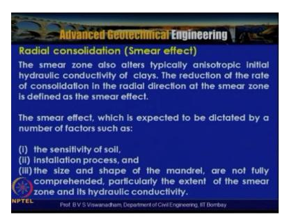
So the smear zone also alters typically the reduction of the rate of consolidation radial direction is at the smear zone so the reduction of the rate of consolidation in the radial direction at smear zone is defined as the smear effect so the smear effect which is expected to be dictated by number of factors such as the sensitivity of the soil and installation process and the size and shape of the man drill.
