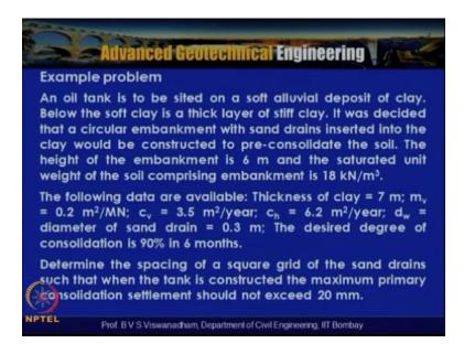
So let us take a problem were the oil tank is to be sighted on a soft alluvial deposit of a clay and below the soft clay is the thick layer of stiff clay so that means that it is actually has got only one way drainage it was decided that the circular embankment with sand drains inserted into the clay would be constructed to pre consolidate the soil the height of the embankment is 6 meters and the saturated unit were to the soils compressing the embankment is 18 kilo meter cube.
