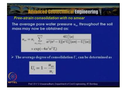
Now the average pore water pressure u average throughout the soil mass may now be obtained as u average is equal to  $u_i \sum \alpha_1$  to  $\alpha_2$  to  $\alpha \infty 4u^{12} \alpha / \alpha^{2*} L^2$ -1 and within square bracket and square  $u_o^2 \alpha_n$ - $u_1^2 \alpha$  and into exponential of you know  $-4\alpha^2 n^2 tr$  so the average degree of the consolidation can be obtained in radial direction has  $u_r$ =1-u average u average by  $u_i$  so  $u_r$  the average degree of
