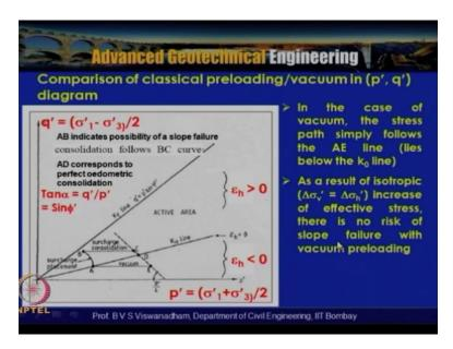
Now another advantage from the stress path diagram we can actually look into the when you take pre loading or vacuum we can see that from p' and q' plots where  $p' = \sigma 1' + \sigma 3'/2$  and  $Q' = \sigma 1' - \sigma 3'/2$  so it can be seen here that in case of a pre loading there is always a possibility that AB is indicating you know the line actually traverses towards the failure line you know AP indicates the possibility of the slope failure.
