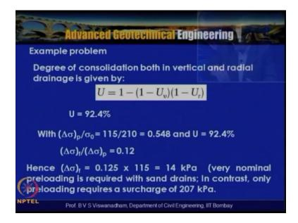
Now after having obtained you know this uv you know 67% and ur 77% by using the degree of consolidation both vertical and radial direction is given by u=92.4% so u=uvr=92.4% and from the given problem we know that  $\Delta \sigma p / \sigma_0$  or  $\sigma f / \sigma_0$  that is from the previous chart here  $\sigma f / \sigma_0$  where it actually shows that it is actually 115/210 that is .548 and U=92.4%.
