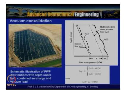
Now this particular slide actually shows the way typically vacuum consolidation is don at the sight so in this what actually has been done is that either with vertical drains it will be much more effective and faster and if you are actually having this drain which is actually connected with you know PDV's and what we need to do is that it actually need to connected to the pump where it actually the surcharge is maintained.
