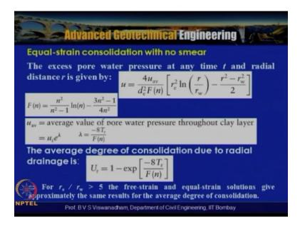
Now the equal strain consolidation with no smear this is actually case for the you know rigid case what we assumed and the excess pore water pressure at any time t and radial distance r given by u=4u suffix average d<sup>2</sup> function of n within sure brackets re<sup>2</sup> natural water of them r/rw  $-r^2-rw^2/2$ teh square brackets close so where fn function of n is nothing but  $n^2/n^2-1$  natural logarithm of n-3n<sup>2</sup>-1/4n<sup>2</sup>.
