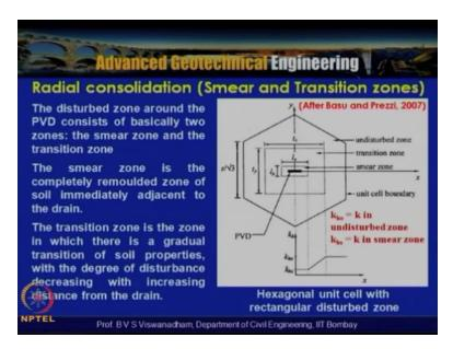
So this is according to Basu and Prezzel 2007 this is for you know PVD's so in PVD's what the portion is that it actually has got you know two zones one is you know three zones basically we can say surrounding the free fabricated drain one is the undisturbed zone that is ever from the drain and transition zone and then you know smear zone.
