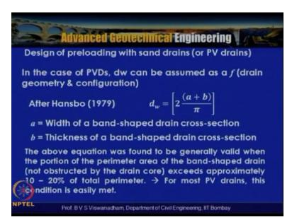
So dw= $2*a+b/\pi$  so this actually has been obtained nothing but you know by equating  $\pi$ dw that is nothing but the you know perimeter of the diameter of the well is equal to 2\*a+b where a is nothing but the breadth of the you know the PVD and B is nothing but the thickness so A is nothing but the breadth of the band shape drain cross section.
