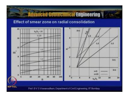
Now here the effect of the smear zone on the radial consolidation is actually given here and this chart is for left side chart is for n and this is for m' so you can be seen that for different values of s=1 s=1.2, 1.5 so this s=1 is that is no smear then with that what we can see that how the m values m' values change and this is actually only for kh/ks=20.
