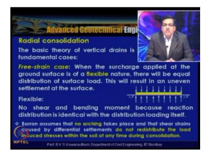
So free strain case is basically for flexible loading like an embankments when the surcharge applied at the ground surface is a flexible nature and there will be equal distribution of surface load that means that whatever the surface load will be there the reaction will be equal and opposite so because of this what will happen is that no bending moment and shear forces will generate and because as there is no the reaction distribution is identical to the distribution loading itself.
