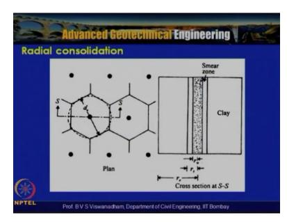
You know the theory is actually originally developed for sand drains but these theories can be extended to vertical drains without much you know difficulties so here this particular horizontal distance which is nothing but Re where two Re is nothing but De or as per our technology it can be capital D=De=2Re so that is the total influenced zone and this is the you know the zone which is actually called form the centre to this one Rs.
