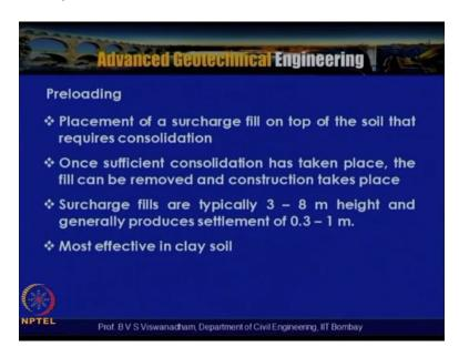
That requires consolidation and once a sufficient consolidation as taken place the fill can be removed and construction can take place that means that if we are having let us say that 10m is the total height including the temporary fill and permanent fill then once the if the temporary fill happen to be three m then the 3m can be removed and left with 7 m so that you know the after the consolidation it can be left with the permanent loading.
