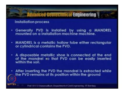
So the installation in the sense that the PVD's are installed by using a MANDREL mounted on a installation machine and MANDREL is a metallic hollow tube either rectangular or cylindrical the cylindrical one which actually contains the PVD. So a disposable metallic shoe is actually connected at the end of the mandrel so that the PVD can be easily inserted within the soil. after insetting the PVD the mandrel is extracted while the PVD remains in position within the ground.
