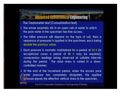
So, the process of the or procedure of the odeometer testing described in the slide the whole assembly with confining ring and the other accessories the with sits in the open cell of water to which the pour water specimen has the access and the initial pressure will depend upon the type of soil then the sequence of pressure applied to this specimen and each being double the previous value.
