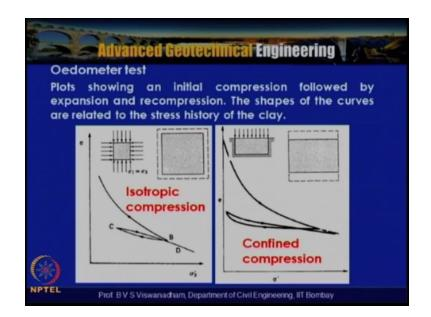
So in the oedemeter test here the first e verse  $\sigma$ ' curves are shown on the left hand side of the slide we see isotropic compression curves where  $\sigma$  1 is =  $\sigma$ 3 the sample is actually compressed in all directions identically so this is this state is called isotropic compression and this is confined compression vertically you can see that this is you know the sample is restrain and along laterally and confined in the vertical direction.
