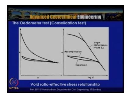
And here is a the result of the odometers test what we get is that we get  $e\sigma$ ' and void ratio effective stress relationships on either arithmetic scale on the logarithmic scale so we can see that initial part is flat and then there is a straight potion which actually coherences here and then once we unload here after reaching certain pressure and the sample undergoes expansion and then the sample is subject into recompression and then goes into the compression mode again here.
