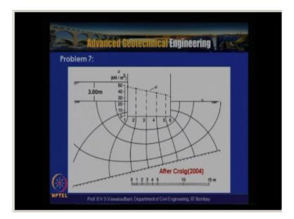
So in the in this slide where the typical flow rate diagram is actually given here for your convenience and this scale is also Shown here and this is the impervious stratum and this impervious this being impervious stratum this becomes the flow line so as you can see that a flow net is drawn with the head of water where here the head of the water which is available for this equipotential line is about three meters by the time it actually comes out it is actually zero so
