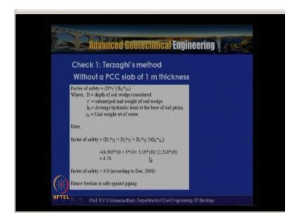
So the check against piping curve one is the check one terzaghi's method let us consider a case of without a PCC slab of1 meter thickness then factor of safety what we have defined is the D into these the depth of intuition into  $\gamma 1$ / HA which is the average hydraulic head at the base of the soil prism so based on that the factor of safety can be obtained with the d1.  $\gamma 1$  - D 2.  $\Gamma$  DT-
