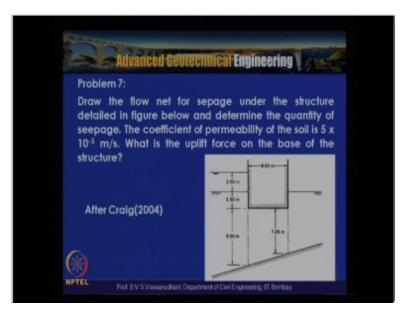
And in the problem 7 wherein we are actually having a situation that we need to draw the sea page under the structure which is the figure which is shown below so draw the flow net for these
