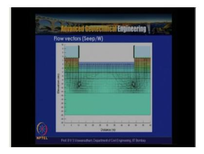
Where in you can see that the trend of flow which a flow line which is actually coming from this direction to this direction so the in order to do the factor of safety against the stability like piping then we required to know they consider a particularly a prism of soil having horizontal distance D/2 and D depth of penetration and then we have to see the factor of safety again is the stability without and with you know the PCC like.
