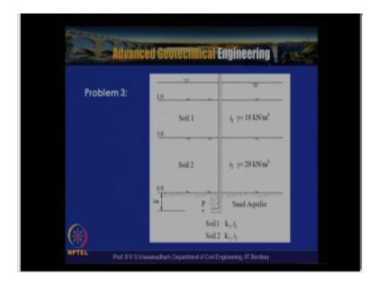
So the cross section of the figure is like this you have got a sand aquifer which is actually having a artesian pressure and here this is this level is 1 meter this is 0 so this soil 1 is having 2 meter thickness soil 2 is having a 3 meter thickness and this is the point P is 1 meter below the soil -bottom of the soil - and here is actually having a hydraulic gradient I 1I 2  $\gamma$  18 kilo Newton per meter cube  $\gamma$  20 per meter cube.
