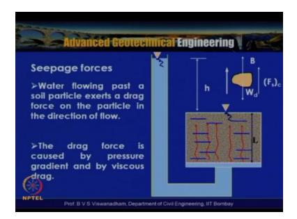
Now we actually have discussed it that when the water flows from higher energy higher head to the lower head, it exerts an energy on soil particles in the process of flowing from higher head to the lower head. So that these particular forces which are actually exerted on soil particles are called as seepage forces. So water flowing past a soil particle exerts a drag force on the particle in the direction of the flow.
