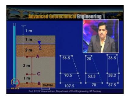
The total stress diagram which is actually shown like 56.5 the units are in  $KN/m^2$  the units are in  $KN/m_2$  56.5 $KN/m^2$  90.5 and or not 7.5 and the water pressure is the thing about 20 and at this point it is 53.3 and 70 and here the effective stress is nothing, but that 6.5 38.2 and 37.5 is having an a constant effective stress of about 37.5 average effective stress of about 38KP.
