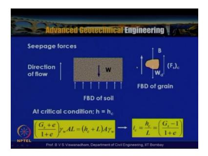
Now further if you look into the equilibrium of an element having cross-sectional area A in the direction of the flow the FBD of the soil is that the weight of this soil mass is W, and the pressure which is actually exerted by the water is actually acting at the base here. So this is the free body of the soil particles or a particle or a grain which is actually shown here. At the critical condition which tends to become HC.
