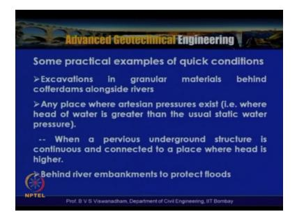
Some practical examples also we discuss there are excavations in granular materials behind the cofferdams along the long side rivers. Anyplace where artesian pressures exist that is where the head of water is greater than the hydrostatic water pressure. Or when a pervious underground structure is continuous and a connectivity a place where the head is higher or behind the river embankments that is levees which are actually constructed to protect floods.
