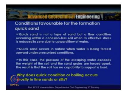
But a flow condition occurring within a cohesion-less soil where its effective stress is reduced to 0 due to upward flow of water. Quick sand condition is not a type of sand, but a flow condition occurring within a cohesion-less soil when it is effective stress is reduced to 0 due to upward flow of water. So quick sand condition occurs in nature and water is being forced upward under the pressurized conditions.
