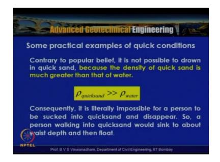
In reality contrary to the popular belief it is not possible to drown in quick sand. The reason is that density of the quick sand which is nothing but a mixture of water and sand particles is much greater than that of water. Consequently it is literally impossible for a person to be sucked into quicksand and disappear. So a person walking into quick sand would sink to about waist depth than the then float okay.
