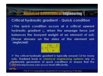
The quick condition occurs at a critical upward gradient I see when the seepage force just balances the buoyant weight of the soil and the shear stresses on the sides of the element are neglected. So here the shear stresses on the sides of the elements are neglected. So the critical hydraulic gradient is typically around one for many soils fluidized beds in chemical engineering systems rely on the deliberate generation of condition to ensure that the chemical process can occur efficiently.
