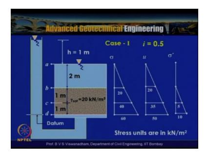
So with this when we plot this diagram with the D, C, B and these points and A at this point, the total stress can be given like this the total stress diagram in units of kilo Newton per meter square can be plotted as 20, 40 and 60. So at this point actually it is 20, 40 and 60 and pure water pressure with the whatever the total heads we have derived we can actually say it is 20 35 and 50 kp so our kp are kilo Newton per meter square.
