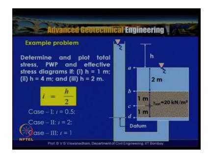
So let us consider another example problem, the problem is described like this here. We need to determine and plot the total stress pore water pressure and effective stress diagram or we need to plot. If incase 1 H=1m, case 2, H=4m, and H=2m. So this is the H which is actually shown here the difference in water level between the this portion of the stem to the this level at a.
