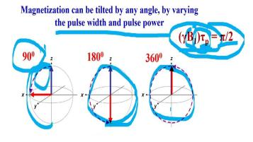
A 90° pulse tips the magnetization to XY
