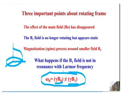
This is how the concept of rotating frame is introducing, and it is very useful in NMR. Now, understand 3 important points about the rotating frame. First point, the effect of the main magnetic field is disappeared in the rotating frame, the spins feel as if B0 is absent, and B1 field is no longer rotating and appear static as far as the spins are concerned, understand.
