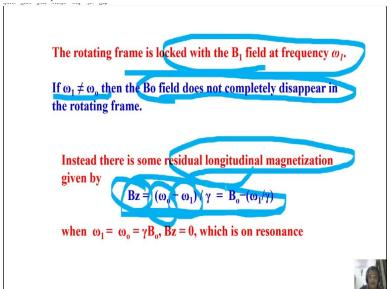
Off resonance condition is the one, where the rotating frame is locked now along with the B1 field at different frequency. omega1 is not equal to omega0. Then what happens? B0 field does not completely disappear in the rotating frame. Earlier when it is exact on resonance, I said the spins freely only B1 field for which B0 main field is 0. The main field is assumed to be absent for the spins, which are processing in the XY plane.
