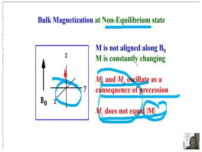
Now, what happens to the bulk magnetization at non equilibrium state? At non equilibrium remember, bulk magnetization and is undergoing precession like this. At equilibrium it was static, Mz = M0. So, now M is not aligned along B0, M is constantly changing. So, Mx and My oscillate as a consequence of precession. Now, Mx and My components I would say is nonzero, in the earlier situation in thermal equilibrium it was in the equilibrium condition.
