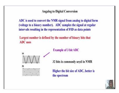
Also we have what is called analog to digital converter. I said signal is in analog mode. But it is collected in a digitized fashion. So, analog signal will be digitized like this. This is analog signal. It will be digitized like this and collected. And ADC is very important. The largest number of ADC is defined by the number of binary bits that ADC uses. For example, if you have a 3 bit ADC, you can have like this. 32 bits is commonly used in NMR nowadays.
