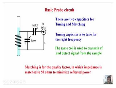
Basically this is a probe circuit. It is nothing but a simple LC circuit, you know. There are two capacitors, tuning capacitors for matching, and the tuning capacitor is to tune for the right frequency. And matching capacitor is to match the impedance, okay. And how do you match impedance? There are two types of impedance matching, which you know in basic electricals. One is 50 ohms matching or 75 ohms impedance matching. I think most of the spectrometers use 50 ohms impedance matching.
