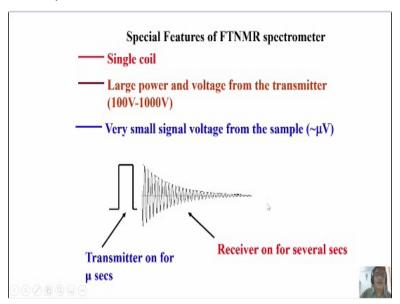
Now, the special features of FTNMR spectrometer. We have a single coil, large power and very small signal voltage from the sample. So, as a consequence, so, we can apply the transmitter for a small microsecond and receive the signal for few seconds. As I said, FID's will be there for few seconds, free induction decay is of the order of 2 to 3 seconds. Now this is special feature of FTNMR spectrometer.
