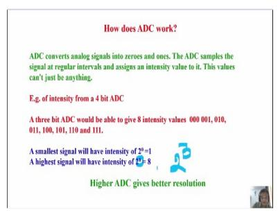
How does ADC work? It is a very simple way. ADC converts signal to digital, coverts analog signal and digitize; and puts into zeros and ones. That is a digit, in a binary digit. 0 and 1 are binary digits. ADC does electronically converts the signal to zeros and ones. And it samples at regular intervals and assigns an intensity value for each of these points, okay. It samples signal at regular intervals and for each of this is, assigns an intensity value and this value cannot be anything.
