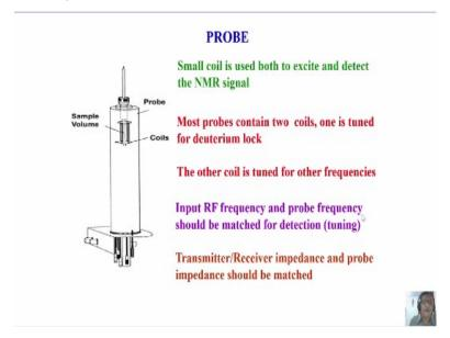
The probe is like this. See inside we have simply a coil here. When you put the sample here, sample tube goes and sits inside this RF coil, okay. The sample sits here. Then using the transmitter, you generate the radio frequency pulse, and to send the pulse. This coil is the one
