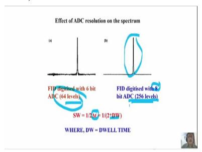
This you will see the advantage of digitization with higher ADC. Comparison of the spectrum it is 6 bit ADC, you have 64 levels. 26 you calculate, find out. This is 8 bit ADC; you have 256 levels, like 3 bit we have 8 levels, like 000 to 111, right. Here, we can have 64 levels; and 8 bit 256 levels. So, we can have a better representation of the signal and higher the levels for representation, better representation of the signal. You can see much better than the 6 bit ADC.
