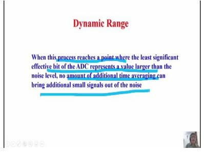
And when this is the thing; what happens? when this process reaches a point, then what happens; when ADC represents a larger value, no amount of additional time averaging can help. The small signals will never be brought out of the noise.
