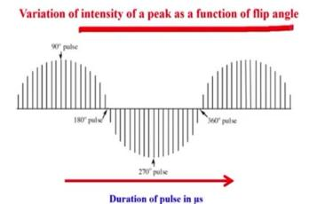
Now experimentally, how it is done? The variation of the intensity of the peak as a function of flip angle is monitored. How it is monitored? Look at this. I have to collect the signal. I take some standard sample. Let us say one which gives me a single peak. I do not know, what is my 180 pulse. I do not know what is my 90 pulse, but I have to calibrate. What I will do is, I will put the sample in the magnetic field, set the pulse width at 2 microsecond or 1 microsecond.
