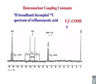
So we can keep on analyzing. I will analyze one simple carbon 13 spectrum with proton decoupling. Look at this molecule, proton decoupled carbon 13 spectrum of trifluoroacetic acid. We have to assign each and every peak here. First, of course, reference is TMS, no need to worry about it. What are these 3 peaks of nearly equal intensity? This is solvent peak, carbon-13 is coupled to deuterium spin 1, three lines of equal intensity, that also is well known.
