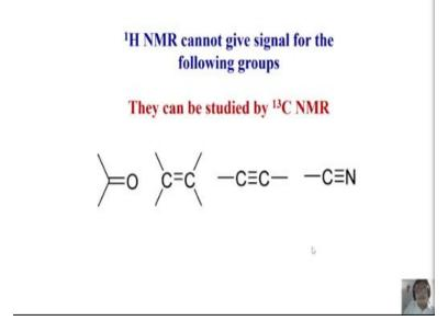
When do you make use of carbon 13 NMR, look for proton NMR? If I have a CO groups; C double bond C, C triple bond C; or CN group like that, if I want to get information about such type of groups present in a molecule, proton NMR cannot give you. Where is the chance for proton NMR to give that information, there are no protons here, and on the other hand I can study carbon here, I can get this.
