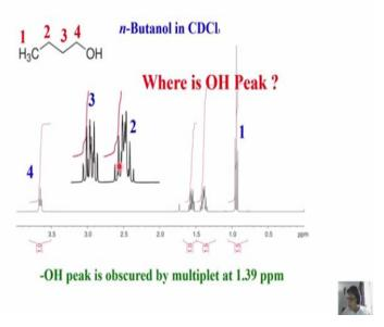
Sometimes you come across a situation like this. It is a very simple molecule I have taken. CH3 CH2 CH2 CH2 OH, n-Butanol; it is done in CDCl3. CH3 you know, it is a triplet because of this. This CH2 is a quartet and a triplet, a complex pattern somewhere here; and this CH2 is a triplet of a triplet because of these two, somewhere here;, and this is a triplet because of this one, that is here.
