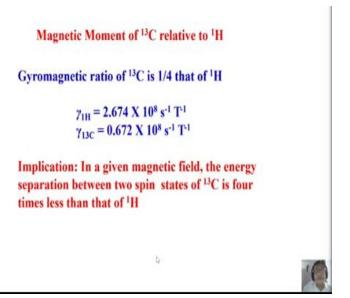
Another interesting point you must know is, the magnetic moment of carbon 13 is relatively four times less than that of proton. That is because gyromagnetic ratio is four times less, I told you. Gamma of proton I said 26.74 into 10 to the power of 7. Similarly carbon is 6.724 into 10 to the power of 7. I told you radians per tesla per second. There must be radians here, it is expressed in radians.
