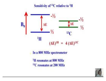
Now this is the energy separation of proton and this is the energy separation of carbon, this is 4 times less. Remember I said, this is also spin half nuclei, okay? This also has two possible orientations; alpha beta. But this is less sensitive compared to this because of less gamma and energy separation is 4 times smaller. I told you about sensitivity when we discussed.
