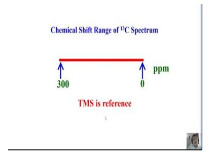
Now, if you look at the chemical shift range of carbon 13, here it is. Measured with reference to TMS, proton is 0 to 10 ppm, but carbon is 0 to 300 ppm, very interesting. Remember, if I have a 500 mega hertz spectrometer, if I want to study proton, 10 ppm, so I will cover only 10 X 500; 5000 hertz. That is all my range of observation. That is the width of spectrum I want to see, called spectral width.
