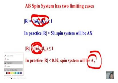
AB spin system has two limiting cases. When this becomes larger and larger the chemical shift separation, compared to J coupling you can take this to AX, that is what you can do. I told you I have a strongly coupled spin system, increase the magnetic field quite a bit, then this becomes
