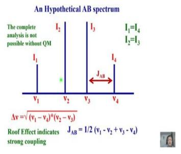
This is a spectrum of AB spin, where A and B are strongly coupled. Look at this one. Are they having equal intensity? No. This is a clear indication of AB and also there is a roof effect, look at it, this is going like this, this is going like this; this is called the roof effect. Remember in the AB coupled case the intensities of the central two lines are equal, and the intensities of the outer two lines are equal.
