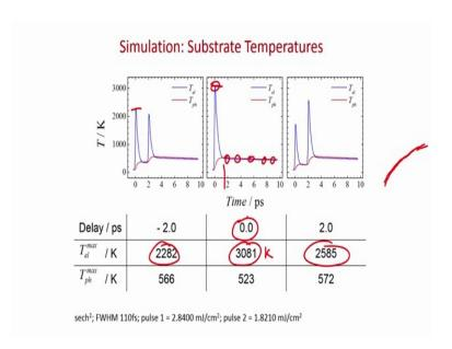
This is an example if two pulses are overlapped together, that is the 0 delay then we see that the maximum electronic temperature is here. This is the maximum electronic temperature. It peaks to 3000 Kelvin temperature its a huge energy transiently we can create 3000 Kelvin temperature. But remember at this 3000 Kelvin temperature, electron and phonon they are not an equilibrium they are out of equilibrium.
