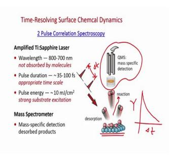
Pulses this is the delta t that is the time delivering two pulses. They will be used to deposit the heat energy on the substrate. And this blue colored surface is the substrate surface and the molecules is desorbing from the surface due to this heat energy dis desorption. And that quadrupole mass spec will be used to detect the molecules which is coming out of the surface.
