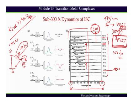
For the experiment a broadband white light pulse it is used to probe the transient absorption that is the way transient absorption spectroscopy is performed. We use white light source and the white light has a band width 440 to 530 nanometers spectral regime and that is why we can monitor the absorption in the entire regime.
