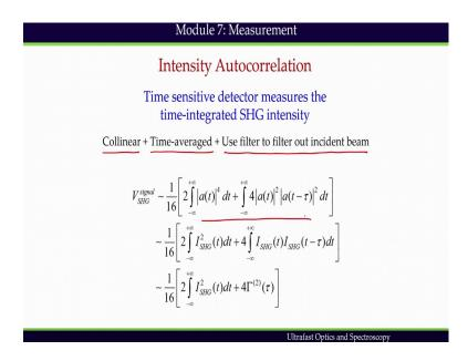
Thus, under correct experimental condition which means we have used collinear configuration, time averaging we have used to suppress other fourth and third terms, and we use filter to filter out incident beam. Under this condition we have only these two terms.
