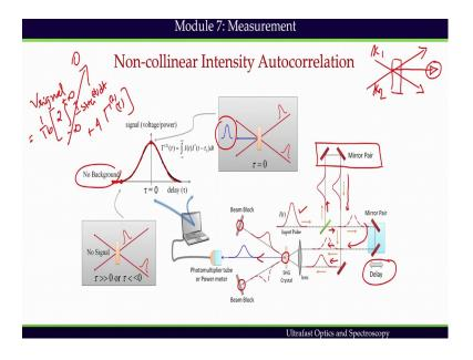
Now, this constant background can be eliminated if we think of non collinear configuration. In non-collinear configuration we have rearranged the interferometer a bit, here we are now using mirror pair. So, let us look at this input beam is split into two by 50-50 beams meter, they go this way the first one goes this way and the second one goes this way, then this is reflected back and this beams also is reflected back.
