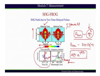
So, one example of SHG-FROG phase is shown here this is two dimensional plot because along this direction we are plotting the frequency wave length along these direction we are plotting delay. At different we are checking the spectrum and the vertical axis is representing the intensity, which means the V's voltage coming out of the spectrometer. It can be easily shown that SHG FROG trace is symmetric function of tau after getting the FROG trace question is how to retrieve the pulse?
