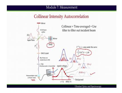
So, if we go back to the intensity autocorrelation measurement we see that the measure second harmonic signal is the sum of constant background. We will have a constant background always at longer delays and the terms which are responsible is individual terms. And an intensity autocorrelation function which will give an enhancement of the signal as long as the two pulses are overlapped which is given by this expression.
