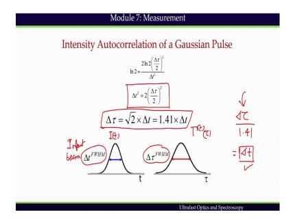
And if we use that then finally, we get an expression which correlates delta t and delta tau, delta t is the intensity full width half max. So, this is your I t profile of the input beam. And this is the corresponding intensity autocorrelation profile and this tau and delta t is now related for a Gaussian pulse it is by the factor of 1.41.
