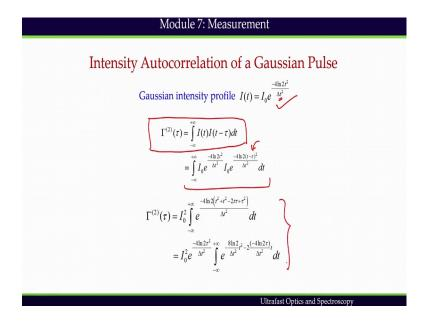
And we will take an example of Gaussian beam to find out how they are correlated. Because then we will be able to use the measurement and predict what was the intensity full width half max of the input beam. So, we take a Gaussian intensity profile which is now very familiar to us, this delta t is representing intensity full width half max we have to emphasize here.
