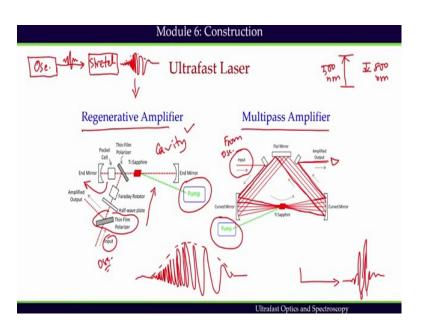
Amplification of chirp pulse is done by titanium doped sapphire, a material having very desirable characteristics, very high damage threshold, high saturation fluence, high thermal conductivity. Therefore, pulses with an energy greater than 1 Joule can be extracted from a relatively small diameter rod, let say 1 centimeter.
