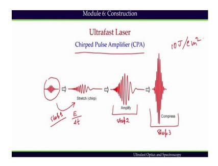
Now, question is if we need more energy what to do? Definitely we have to amplify the pulse. Due to this high peak intensity ultrafast pulses cause local heating at the bulk or surface of the gain medium resulting in thermal fracture, decomposition, melting of the gain medium. The surface damage threshold; however, varies based on thermal diffusion, how quickly the local heat is dissipated over the bulk of the optical element.
