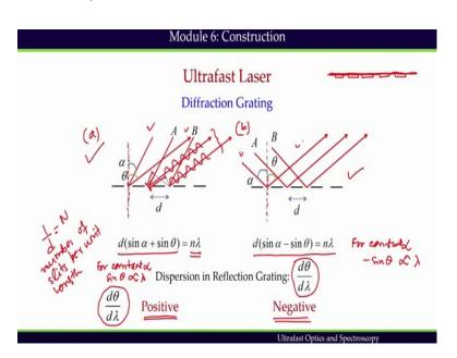
But we will discuss this shortly, before we do that we have to go over the grating equation; need to understand the property of a grating. A diffraction grating is an optical element that possesses an arrangement of a large number of parallel equidistant and closely space slits of same width which are placed side by side. If I have a flat surface we prepare slits like this, we make grooves and the surface becomes grating surface.
