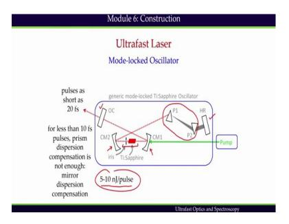
We have dispersion compensate dispersion compensator given by two prisms, high reflector. We have self phase self mode locking done by this aperture and the gain medium and the laser cavity with the help of these two mirrors and the output coupler. So, this kind of laser oscillator this kind of ultrafast oscillator can produce energy in the range 5 to 10 nano Joule per pulse.
