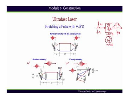
But before injection into the amplifier short pulse needs to be stretched in time by introducing a frequency chirped into the pulse which increases the duration of the pulse by a factor of 10 to the power 3 to 10 to the power 4. The duration of the stretch pulse is determined by the damage threshold of the optics and non-linear distortion of the spatial and temporal profiles of the beam.
