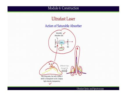
Saturable absorption is a property of any material where the absorption of light decreases saturates with increasing light intensity or in other words transmission of light increases with increasing intensity of light passing through it. At sufficiently high intensity of the input beam ground step population is depleted completely and therefore, absorption saturates and the material becomes transparent at high intensity.
