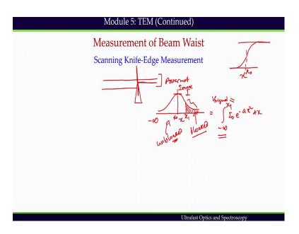
We obtain a curve similar to the one depicted in this figure. This kind of curve we obtain in this measurement as a function of x and this is x naught. And, as many laser applications we use Gaussian beam TEM 00 more we use the power detected by the scanning edge measurement can be easily estimated from the area under a portion of the Gaussian function.
