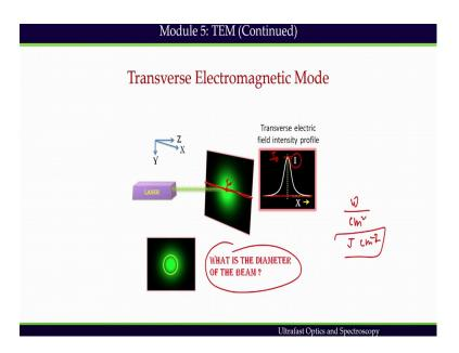
And, we have already pointed out that rays are idealized or oversimplified model of the laser beam. In reality a laser emits a beam of finite width or diameter. If a piece of paper is placed on the laser beam we get the cross sectional area illuminated by the laser beam as shown here. What you observe is called transverse electromagnetic mode of the laser.
