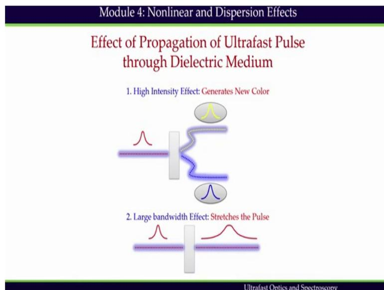
Welcome back to module 4. In this module, we will continue more discussion on Nonlinear Effects and Dispersion Effects, which originate due to propagation of ultrafast pulse in dielectric medium. We have seen already that when an ultrafast pulse propagates through dielectric medium, it experiences both nonlinear and dispersion effects.
