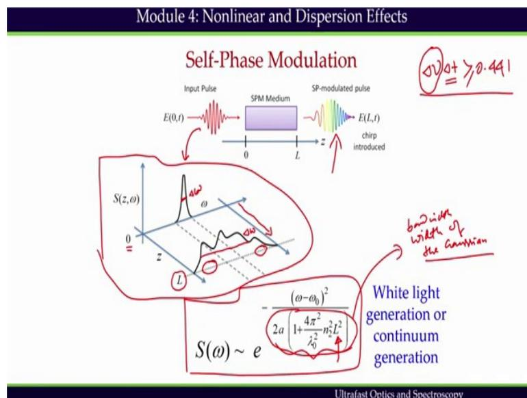
So, here we are interested in the shape of the power spectrum we can consider only the real part and the normalized maximum amplitude and we see that the power spectrum has an expression like this, which suggests that this denominator in this expression in a Gaussian function defines the width of the Gaussian. So, basically this is defining the
