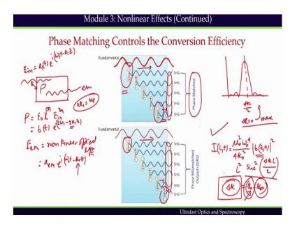
So, this is at 0, if you plot delta k l by 2 then we get. So, cardinal sine functions will be like this, very sharply it drops down its maximum when delta k equals 0, this is maximum and it drops down very quickly when there is a phase mismatch. So, this delta k issue bringing them in phase we have to consider for the HHG process as well. ( <u>look the slides for mathematical expressions</u>)
