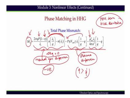
So, this neutral gas dispersion instead of positive this, this term becomes negative. The second term which is plasma dispersion on the other hand is positive because q is greater than 1 by q. So, this is negative so this negative is contributing to this negative. So, finally, this is becoming a positive contribution.
