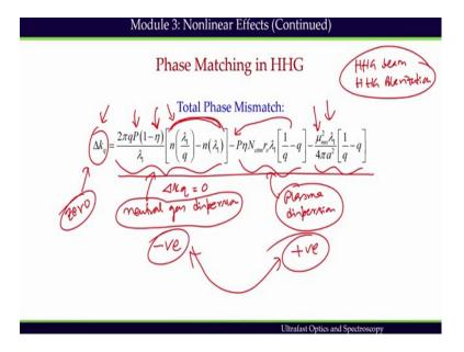
When an intense laser beam interacts with the gas medium, free electrons are emitted. These free electrons cause plasma dispersion, as the contribution from the phase mismatch due to neutral gas dispersion is negative and due to plasma dispersion is
