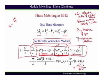
P is the pressure of the gas medium and  $eta(\chi)$  is the ionization fraction and n atmospheric it is number density at 1 atmosphere it is the number density in 1 atmospheric pressure and n lambda is the refractive index of neutral atoms. (look the slides for mathematical expressions)
