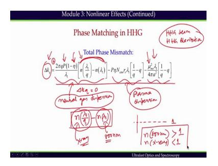
So, the phase mismatch which we can write like this way by this expression and this expression gives us the phase mismatch between the emitted beam HHG beam HHG beam and HHG polarization that is that is going to control the phase matching. The phase mismatch can be given by this which has this expression here waveguide contribution we have included, if we are not using waveguide then we can we can remove this contribution.
