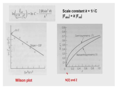
Here is the expression given logarithm of I relative by sigma, i going from 1 to n and so, we get this expression and this is like y equals n x plus C equation. So, when we plot this logarithm value against sin squared theta by lambda squared, we will be ending up getting a straight line; the intercept is log C and the slope will be corresponding to 2 B.
