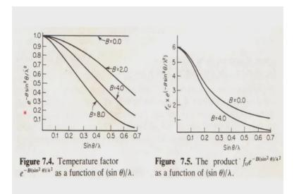
For example, if we put now e minus B sin squared theta by lambda square on the y axis, plot it against sin theta by lambda. As the value of B increases, of course B equals 0 will be very constant. There is no thermal parameter associated with it, but that is not very ideal case which is impossible case. In fact, because the atoms are always moving they are not at rest any time. So, as the B value increases you notice that this value which is e
