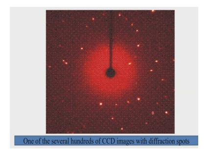
The purpose of this is to see what happens when we do the diffraction. So, we do the diffraction in this one of the CCD images which shows the reciprocal lattice images. So, these are the reciprocal lattice points which are seen here dark and white. We know why some of them are dark and some of them are not so very dark as are bright as we have seen from our positioning of the atom with respect to the planes.
