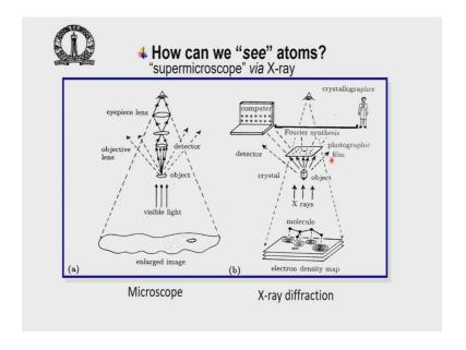
So, as we saw earlier also this slide that it is taken from the book of Glasker and Tubuler it is a old book and that is how we have now shown here a photographic film in that place we put now the CCD camera or the CMOS detector. So, what essentially it does is comparison between a microscope and a x-ray diffraction experiment. In case of a microscope the object now sends scattered radiation. Here the radiation is following the Braggs condition because it is a crystal.
