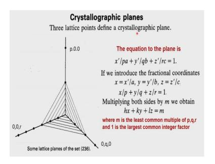
So, having learnt what crystallographic directions are we will now go to the crystallographic planes. In case of a crystallographic planes we need 3 lattice points the diagram below is shown here it represents the 2 3 6 that is because I have shown two along this direction 2 units and then you see the lattice points two are along these direction and here it is 1 2 3 4 5 6 along the vector r along the vector p it is 2 and along the vector q it is 1 2 and 3.
