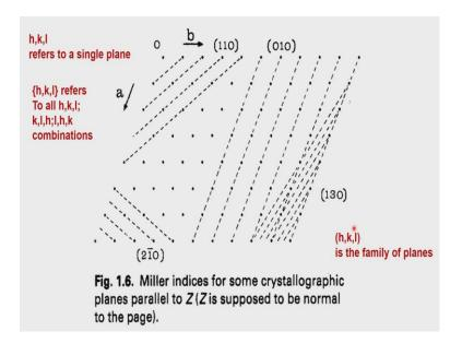
We can generalize it a little more by looking at this diagram. Now this diagram tells us that we have a lattice this is the 0 point and these are the lattice points along the a direction and these are the lattice points along the b direction and these are the lattice points which define our unit cell.
