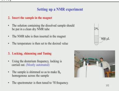
You can see that what typically is done is the first you take the sample in a clean dry NMR tube and this is shown on the right side. This is typically the picture of NMR tube here, it consists of 5 mm diameter glass tube and this is 5 mm diameter it can also be smaller 3 mm and depends on the spectrometer, the standard overall you everywhere is basically using a 5 mm NMR tube and the sample volume, which is shown here the sample exactly about 600 micro litres.
