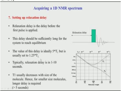
Another next important parameter to setup in a 1 D NMR experiment is what is called relaxation delay. So, if you can recollect in the last class we showed you the pulse sequence. A pulse sequence is basically a diagram a picture of how the different pulses are executed in NMR experiment and one of the first it consist of pulse sequence basically consist of pulses and delays. So, R F pulses and delays.
