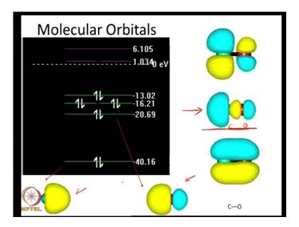
So, here I have just reviewed for you all the orbitals, which are of importance. This is the sigma orbital, which donates electron density. You will notice by looking at the 3 sigma orbitals. This is the first sigma orbital. This is the second sigma orbital. This is the third sigma orbital, which is the highest occupied molecular orbital. The number of nodes between the carbon and oxygen keeps increasing.
