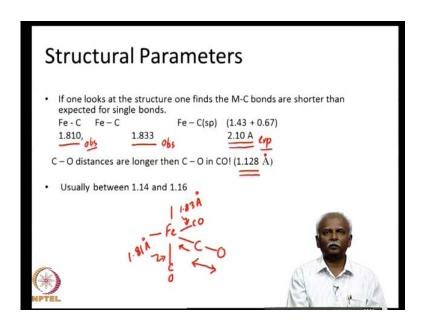
So, let us proceed further. Let us look at just and revise some of the structural parameters that characterised the metal carbonyl compound. If one looks at the iron carbon bond in an iron carbonyl complex, we noted the fact that the bond distances should have been approximately 2.10 Angstroms. This is the expected value. What we observe this is the observed value. So, very clearly, the observed value is much shorter, either it is 1.833 or it is 1.810. These are two observed values in a complex.
