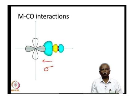
So, the first important combination is donation of electron density from the carbon monoxide. So, carbon monoxide gives a pair of electrons to the metal. As I mentioned before for convenience, we have only pictured the d x square minus y square orbital. But, it is actually a hybrid of the d s and 3 p orbitals. So, this hybrid accepts electron density from the carbon monoxide.
