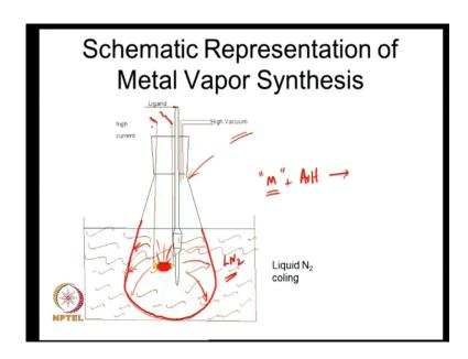
So, this turns out to be an extremely general method. Here is a schematic of a schematic diagram of this setup. You have a way to vaporize the metal under very high vacuum this whole reaction vessel is kept under very high vacuum. And that temperature when you have a very high vacuum, you can now pass the ligand, so that the ligand is now quoting the sides of this vessel.
