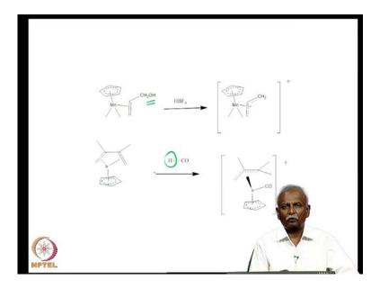
Now, we if you remember the preparation of allyl molecules we used two different types of preparations. Two major classes of preparations one of which was a case, where we took the allyl alcohol coordinated to a manganese for example, and treated it with HBF 4, HBF 4 is a strong acid. It converted the OH group to a positively charged system, and it generated a water molecule and an at least an allyl cation. Which is coordinated to the many is, but because of our electron counting nomenclature.
