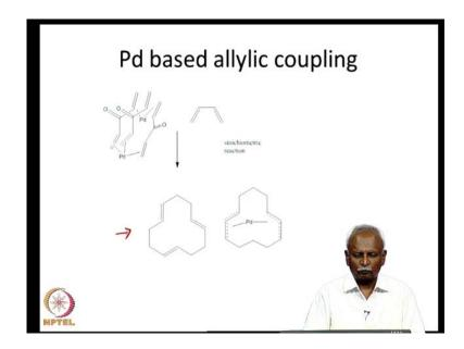
So, the same reaction if the reaction is not done in a stoichiometric fashion, it could be done in a catalytic fashion, and one can isolate the cyclododecatriene. So, this cyclododecatriene is formed by the carbon carbon coupling action, that we just discussed and it is formed as a result of stitching together three molecules of butadiene.
