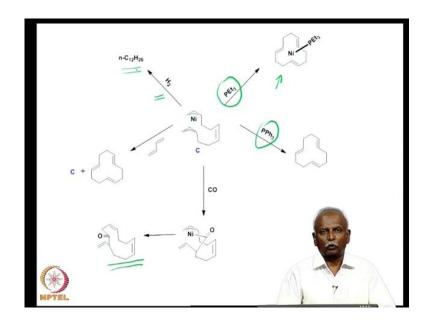
If you use carbon monoxide, he showed that you can in fact do a reductive elimination where you have one CO, which is inserted in during the insertion process. Then that seems to be fairly understandable if you use a high-pressure carbon monoxide, you can introduce a carbon monoxide instead of adding another molecule of butadiene. So, that is what is happening here, so you get a ketone and as one of the products.
