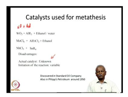
So, what we have not discussed in the last lecture where we discussed the mechanism of this process is a fact that the catalysts required for the metathesis were often very complex. Originally, it was discovered by the standard oil company and patented also by Phillips petroleum for a specific case. Most of these companies used very complex mixtures for carrying out metathesis.
