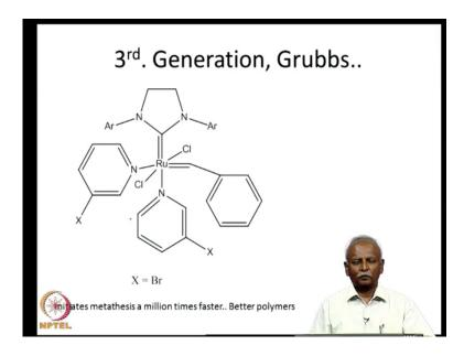
Grubbs showed that if you replace the pendant group with a peredene unit a substituted peredene. If you react the Grubbs second generation catalyst with a peredene specifically, bromo peredene then it turned out to be an extremely useful catalyst it was extremely reactive. In fact, it initiates metathesis a million times faster than the second generation catalysts this like I said earlier it turns out be an extremely important fact for polymerisation.
