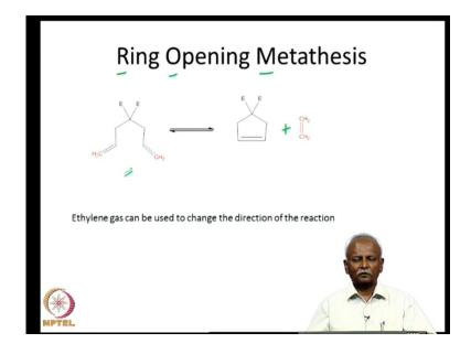
Now, you will notice that the same reaction can be pushed in the opposite direction if you have a large amount of ethylene. Suppose, I have a high concentration of ethylene and I take the ring closed product, then I can have a ring opening metathesis. So, this is called RON the previous one is called RCM and this one is called ROM, and the ring opening metathesis can push the reaction from the ring closed system to the ring open system.
