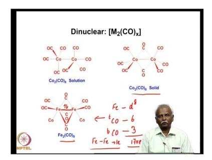
So, here I have pictured the two structures of the dicobalt octacarbonyl complex. In the dicobalt octacarbonyl complex in solution, you find there are no bridges and in the case of the solid state structure you have a very clear formation of a you have a very clear indication of a bridge structure. In the case of dicobalt monocarbonyl that is Fe 2 C O 9 you find that the 3 triple e-bridging structures and that in that involve the necessity of a metal-metal bond.
