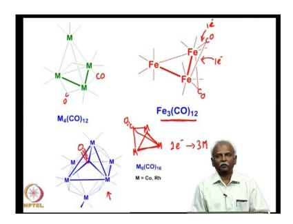
Here, I have pictured a series of trimeric and tetrameric species and in each one of these systems you will encounter a bridging carbon monoxide. In some cases it is bridging 2 metal atoms in this case. For example, it is bridging 2 metal atoms and so we have pictured it as the vertex of, we have pictured it like this where the 2 lines meet that represents bridging carbon monoxide. In other systems where 3 lines meet you have a triple e bridging carbon monoxide.
