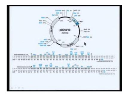
And you can see, the pBR322 was almost about 4 kb, whereas the pUC 19 is only about 2.6 kb. So, the vector size is much smaller, and therefore, larger plasmids can be cloned into pUC. It had an ampicillin selection marker for selection, for antibiotic resistance. This is the detailed map of the pUC plasmid. As I said, the multiple cloning site contained a number of restriction sites here.
