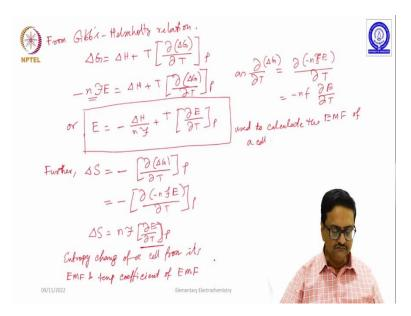
So, now, from our knowledge of basic thermodynamics we know from Gibb's-Helmholtz relation delta G is equal to delta H plus t del delta G del T at constant pressure P. So, now, we replace this delta G by n f E that is minus n f E which is equal to delta H plus T as it is del delta G del t P. Or simply one can write E equal to minus delta H by n f plus T del E del T P as del del T delta G is nothing but del minus n f E by delta t or minus n f del E del T.
