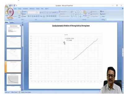
I have taken the line on after the equivalence point which is showing a steady increase in the conductance and in the same way I have drawn a best fit straight line using this data points and again it is 0.998 which is again a good fit. So one can easily calculate the endpoint by using these two equations.
