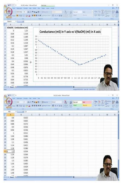
So what you can see here is that I am demonstrating it with the data of strong acid versus strong base titration that is HCl versus NaOH. So in that experiment, we generated the data with different volumes of NaOH and the corresponding conductance in milli-siemens that was recorded.
