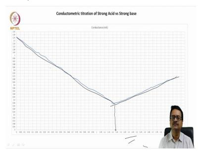
The other method using graph paper is for you to draw a straight line, draw a straight line from this to that using a scale and then also draw another straight line using those. Wherever those two straight lines meet that will be your equivalence point.
