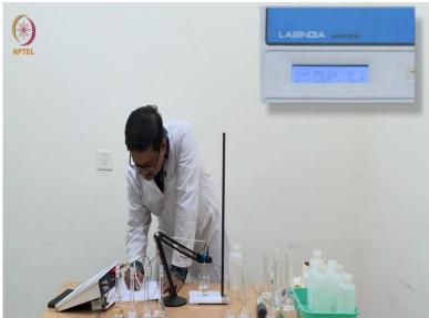
So now I am going to use this N by 4 acetic acid for my seventh reading and then we will end with N by 2 acetic acid. So now you will see the number has jumped to 932 and it is still increasing. We need to wait for a while for the meter to stabilize. Maybe 932.7, 932.7 is probably the reading, still increasing. So we take this as the reading, 952.2.
