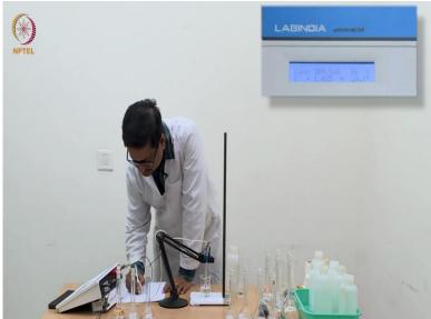
Now I am going to use this N by 32 acetic acid solution for conductance measurement. So now we have doubled the concentration from N by 64 to N by 32. The conductance has increased from 204 to about 310. It is now trying to stabilize around 309.7, 309.6.
