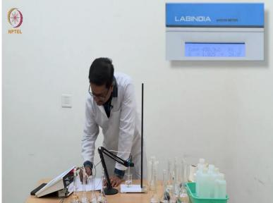
Now I will use this N by 16 acetic acid solution. I am taking this reading as 458.9. Remember that we are still in the micro-siemens range which you can see from this reading.
