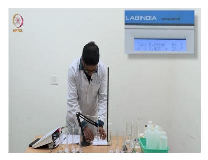
Now with distilled water, you can see that it is reading about 8-9 micro-siemens so that means the electrode is almost clean and one can use this electrode once again for any further experiment. So with this, I conclude this experiment and we will meet in the next class with the results and graphs of these experiments. Thank you.
