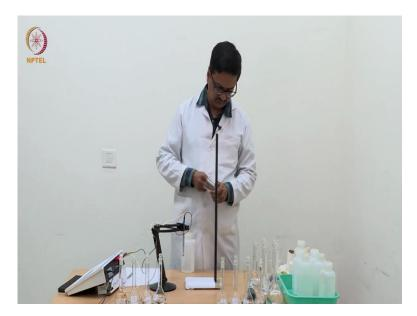
So we first wash it again with a lot of water and discard that water 2-3 times and then make sure that the conductance of water is read below 10 micro-siemens.
