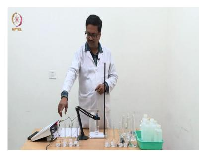
So I have used this 1 normal acetic acid solution to prepare N by 2 acetic acid by half dilution, from this I have prepared the third solution N by 4; like that we have come up to N by 256 by half dilution method. So every time I have taken 50 ml of the solution and diluted it to 100 ml to make it half diluted.
