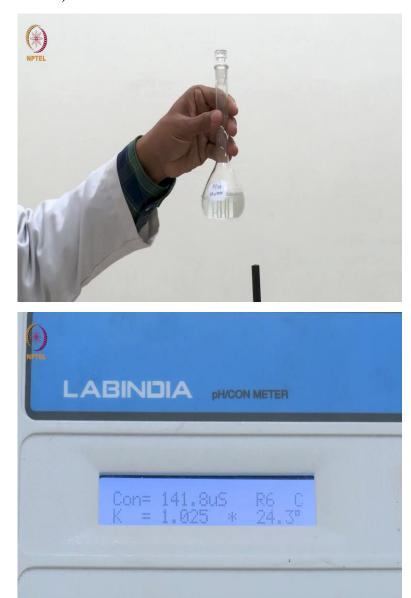
Now I am adding this N by 128 acetic acid to this beaker and we will measure the conductance. So it is 141.9 micro-siemens.
