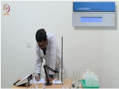
Now I am going to use this N by 64 acetic acid and measure the conductance value. So with this N by 64 I am getting a reading of 204.2. Already you can notice that the increase in conductance with increase in concentration every time two times, the conductance is not increasing two times which was happening with HCl.
