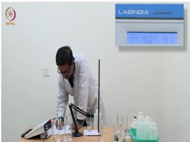
This is the sixth solution with N by 8 concentration of acetic acid. So I am going to use this now. What we are seeing is that there is, the increase in concentration, with increase in concentration, there is increase in conductance but it is not doubling or it is not a regular curve, change concentration which indicates that it is not a linear change.
