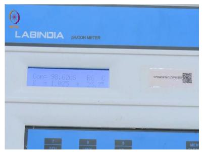
I am going to use this N by 256 acetic acid solution to start with, and then slowly I will go ahead with more and more concentrated solutions. Since I had just water first time, I am just going to wipe water with tissue paper and remove the tiny trace and also dry this beaker with tissue paper to remove any trace of water which may then also further dilute the acetic acid which I am going to pour here.
