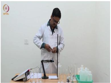
So we will now change this with the N by 128 that is double concentration. So we put it back. We need to wash the electrode once with water as before and we will then use the next solution and measure the conductance.
