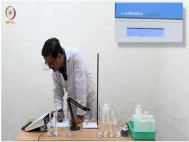
Now I am going to use this N by 64 HCl solution and then get its conductance value. So with N by 64 HCl, we are getting a reading of 7.727 milli-siemens. So with continuous doubling of concentration, we are getting nearly double the conductance value.
