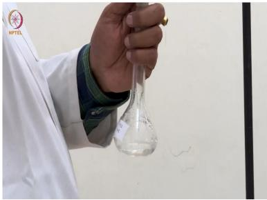
So let me start with this 1 normal HCl solution. This experiment will depend very much on the accuracy of this dilution because here if we make a mistake in dilution if we take little more or little less, the concentration will be different. As a result, the measured conductance will have a significant effect.
