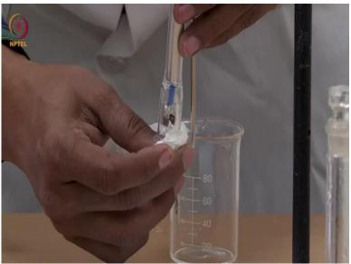
So now I am going to take the most dilute solution which is N by 256 concentration of acetic acid. Transferring a sufficient amount so that the conductivity cell, the electrode is dipped and what we see is that you get 1.7, 1.8, 1.9. So let it stabilize, we will take the reading for this. So we have n by 256 hydrochloric acid and the corresponding conductance that I am getting is 1.771 milli-siemens.
