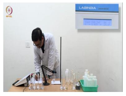
As I am now reaching higher concentration, this cleaning has to be done very carefully so that no drop of previous concentrated solution stays here because every drop of that solution may result in a change in the conductance in terms of 1 or 2 milli-siemens.
