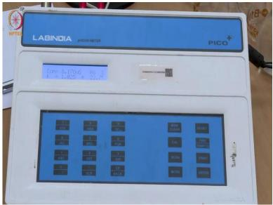
In this particular page, I am going to take the reading. You can see the dilution that I am going to do. I have already written down the conductance of the solution water which is slightly changing. It is like 1.17. When I noted it was 1.14. This value actually does not make any difference because when we add this acid solution whether it is acetic acid or HCl, we will see the conductance of that solution.
