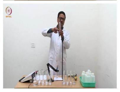
So now I have transferred 50 ml of 1 normal HCl in this and carefully I will add water to dilute it, to 100 ml. Towards the end, one has to be very careful to make sure that there is no air gap or air bubble in the volumetric flask which will then result into a slight change, decrease in actual volume.
