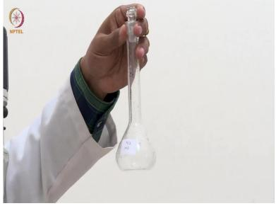
How are we going to prepare these dilute solutions? We are going to use a 50 ml pipette with a pipette pump here. So this 50 ml pipette we will pipette out 1 solution. We will start with 1 normal solution which we will take 50 ml, transfer it to a volumetric flask which is marked as N by 2.
