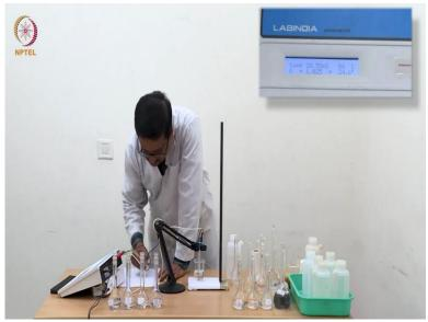
Now I am going to use this N by 16 HCL. I am slowly increasing the concentration as you can see and the conductance value is also significantly increasing. Every time it is becoming nearly double. So N by 16, the reading is 28.56, 28.57 like that.
