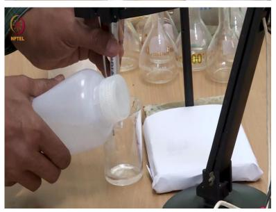
So now I am pouring this N by 128 HCl solution. So this is a double concentration. So you should see a significant increase in conductance of measured using the electrode. So with 1 by 128 normal HCl, the reading is coming as 3.74, 3.740 milli-siemens.
