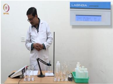
Now I am going to use this N by 32 HCl solution and get the reading. So every time you can see that when we are cleaning and taking it back, the reading is going back to about 8 to 9 micro-siemens and now I have added N by 32 HCL. It should read maybe nearly double of what we had seen before. It was 7.7 and now it is about 16.5, 15.8 and it is stabilizing at 15.86.
