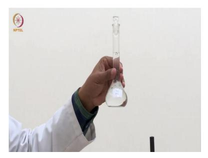
So after taking it up to the mark, we close it and shake well to homogenize. So now this solution is a homogeneous solution of N by 2 HCl. So with this N by 2 HCl, we will now prepare N by 4, and then from N by 4 we will make N by 8, and so on.
