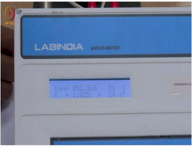
So, now I have reached a 0.1 ml and I should mix well so that the solution is homogenized. We will see that little more precipitated has formed and the solution is becoming more non transparent with time, but the conductance value it is not changing at all, it is still remains 852.2. This indicates that our experiment is going in the right direction.
