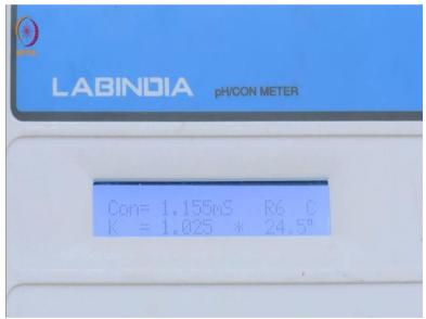
We will take one more reading with 2 ml and we see that this is coming out to be 1155 millisiemens, micro-siemens. So, now if you see beyond about 1 ml which is just after the equivalence point the conductance was increasing. After 1 ml it is 1.25 is 85 from 885 to 978 is about 90, 978 to about 1,073 is again about 80. So, this constant increase 80 to 90 millisiemens, micro-siemens indicates that we have got 3 or 4 points which are after the equivalence point.
