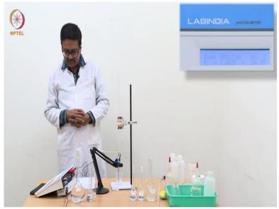
Now, we will keep on adding 0.25 ml as before and take the drop in solution, mix well, shake well. So, now what is happening is all the chloride ions are consumed, whatever we are adding we are adding AgNO3 and the conductance increasing is corresponding to the amount of silver plus and nitrate ions that are added on top of whatever ions were present in this solution from the very beginning.
