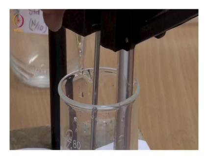
So, we will now keep on adding 0.25 ml each time and take the reading. So, now we have reached 0.5 ml and the reading is slightly reduced, but then again it will equilibrate and give you approximately the same value as you know the conductance of chloride and nitrate is about the same. It is not exactly same and that is why we are seeing a slight gradual decrease. So, it is 842.6. We will add another portion of point, this burette is different.
