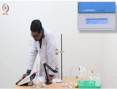
So, now I am going to pipette out this triple mixture and add it to this water for the estimation. As soon as I start adding this solution you will see that the conductance of the solution is changing, it will be increasing. So, it will take a while for the instrument to stabilize and equilibrate to the correct conductance of the solution which is solution of triple mixture.
