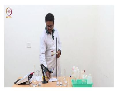
So, at the moment what we have taken in the beaker here is just some amount of distill water and you can see the conductance of that distill water is shown here it is about 8 microsiemens, 8.72 micro-siemens.
