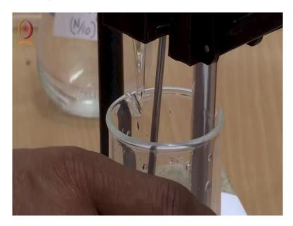
We will add one more portion of 0.25 ml. So, we compare to the previous experiments of both potentiometry and conductometry here our step size is more because we are in a region where we are expecting a nearly flat straight line where the conductance is not decreasing significantly. You see that we have already added 1 ml of silver nitrate and the conductance is now showing here in the conductivity cell it is 829.
