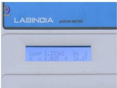
And we will just for the safety purpose we will take one more reading with another addition of 0.25, so we have 2.25, because at the end when we try to plot we should not be following short of the number of points. One or two points may go out of the straight line so we would need about 4 to 5 points to draw a best fit straight line. So, with 2.25 it will stabilize and give us the reading in a while.
