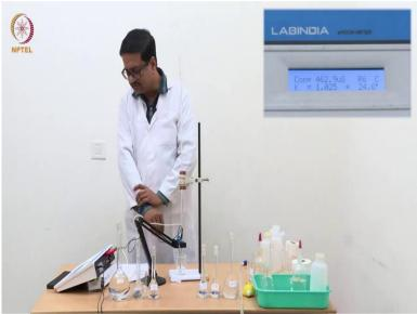
So, with 0.68 ml the reading is 454, maybe it will reach 455, if we wait and let it homogenize and equilibrate because at this point the neutralization has just happened and if the instrument also takes a while to read the conductance very accurately.
