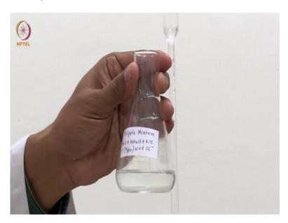
So, in this particular experiment I have prepared an unknown solution of a triple mixture which you can see is a mixture of hydrochloric acid, ammonium chloride and potassium chloride and the overall strength of this solution in terms of chloride is approximately N by 100. So, we want to use conductometric method to estimate the concentration of individual components that is HCL, ammonium chloride and KCL.
