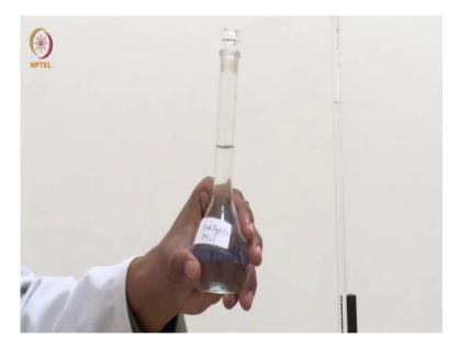
Then we have to discard the solution, take the fresh solution of this triple mixture which is mixture of HCL, ammonium chloride and potassium chloride and we will then titrate that mixture using a standard silver nitrate solution which we have prepared again using the very accurate weighing method, using weighing bottle and the 4 digit balance. So, this is a standard N by 10 silver nitrate solution.
