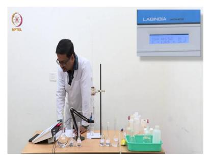
Now we have reached 0.24 ml and the conductance is 548.2. So, again about 40 microsiemens decrease in conductance. So, with 0.28 we are now close to the... What happened, it is not reading. So, the electrode was above the water level, so it was not reading the correct value, we should wait for it to stabilize and homogenize as well. So, then you know that we are close to the neutralization point.
