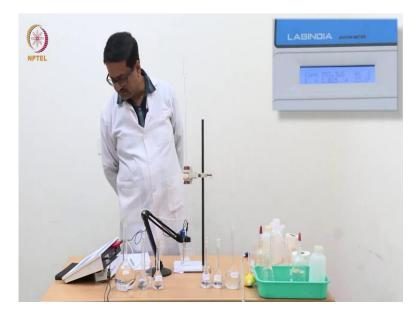
So, now what we have in your screen, we have a solution of 0.01 molar KCL and the conductance that is reading here is 1.441 milli-siemens with a cell constant of 1.025. So, we will require the value of cell constant in the calculation.
