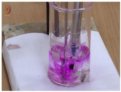
We will just add one drop of phenolphthalein in this solution to make sure that whether we have crossed the equivalence point or not. So, now I am adding just one drop of phenolphthalein to see whether we have crossed the equivalence point or not. So, now you see that the solution it has turned pink. So, this reading of 0.80 which is 211.6 is a point where we have crossed the equivalence point, maybe in the previous itself we have crossed that we will know when we plot the graph.
