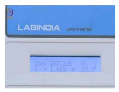
So, now I had added 1.1 ml reached 90.90 and the conductance has increased and stabilized quickly to 67.2. You see when it is just NaOH and there is no hydrolysis, there is no disassociation of acidic acid the conductance is reaching its equilibrium value very soon. So, this certainly is of course an indicator we did not have to add the indictor to know whether we have crossed or not.
