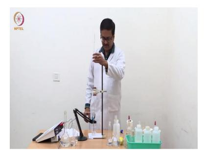
So, using this burette I will be adding 0.04 ml portion of NaOH and measure the conductivity and note down the readings. Now I have added 0.04 ml of N by 10 NaOH which is nearly 10 times strongly than the concentration of acidic acid and the conductance has reduced to 60.77.
