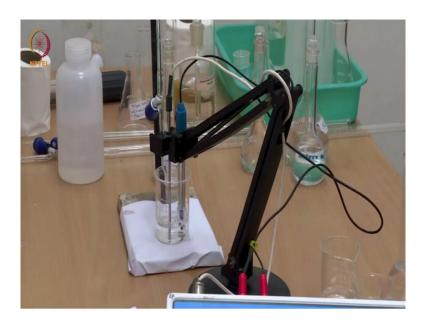
Now, we will take about 20 ml, 25 ml of water such that the electrode is completely dipped in water and it should then show the conductivity of this water which should be close to about 8 to 10 micro-siemens. So, you can see in this conductivity cell, the conductivity meter you can see the reading has come to about 8 micro-siemens which is fine for a good quality distilled water because when we add acidic acid the conductance of this solution will increase.
