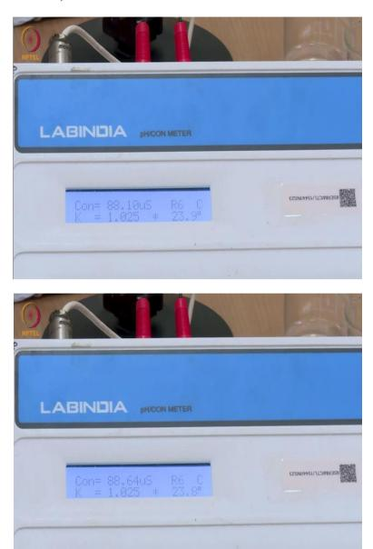
You see basically initially the conductance falls much below every time we are seeing the same phenomena and this is nothing, but due to the consumption of H plus by NaOH that we have added, and then slowly acidic acid disassociates, and compensates for the consumption of H plus, so the equilibrium is reached. And we are reaching a conductance which is now the equilibrium conductance of disassociated acidic acid along with some Na plus ions. Now, we have reached a stable value of 88.64.
