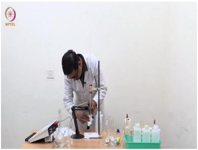
Now, I am going to change the solution, I am going to keep this KCL solution aside and before doing anything I need to wash the electrode thoroughly so that there is no leftover KCL in the electrode, wash it with plenty of distill water, wash the temperature sensor and discard that water then we need to wipe it out once with tissue paper to remove any water droplet.
