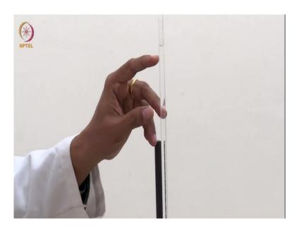
And we will use this N by 10 acidic acid as the unknown analyte, this is prepared approximately N by 100 and we will titrate this with the stronger, 10 times stronger NaOH solution which is N by 10 NaOH which I have taken in this 10 ml burette which you can see here is a 10 ml burette and I have filled it up to the mark.
