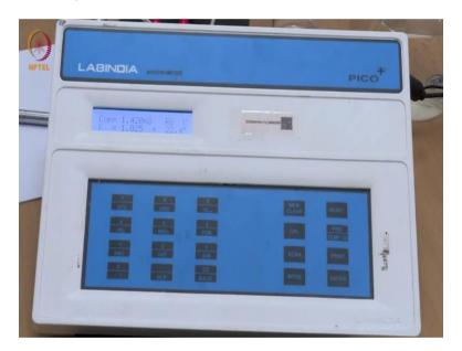
So, here you can see in the inset that I have already calibrated the conductivity meter with a solution of 0.01 molar KCL and the conductance of that 0.01 molar KCL is supposed to be about 1.4 to 1.44 milli-siemens with a cell constant of 1.025. So, with this solution we have calibrated the instrument. Now, I will change the solution I will keep it aside for future checking once again after the experiment is over.
