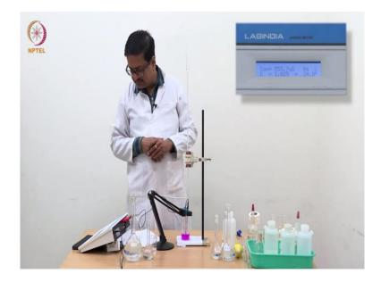
So, let us just wait for 10 seconds to let this conductivity meter stabilize and show me the final conductance of this solution and we will note down the value as 553.8. So, with this we come to the end of this titration of weak acid versus strong base using potentiometry. So, here what we have shown, we have seen from the reading. When we plot it will a evident, we start with a particular conductance.
