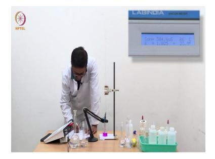
So, we have reached 1.1 ml and the conductance is 384.6 we will go to 1.2 ml. You see that after adding the conductance has not changed because it has only changed the conductance of the locality where the drop has fallen and then when I shake, when I try to equilibrate, when I try to make it uniform, homogeneous solution then the effect of additional NaOH is easily seen in the conductance of the solution.
