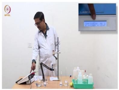
You see now I am going to clean the temperature sensor and also the outer part of the electrode carefully without touching or without spoiling the electrode with the tissue paper
