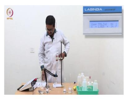
Now we have reached a value of 0.6 ml of NaOH added and the conductance that we see here is 0.778 milli-siemen or 778 micro-siemens that you can read from here. So, for our simplicity purpose we should always maintain the same unit although the instrument maybe showing in a different unit because it shows with 3 decimal places and then there is 3 significant figures and then after decimal you have one figure.
