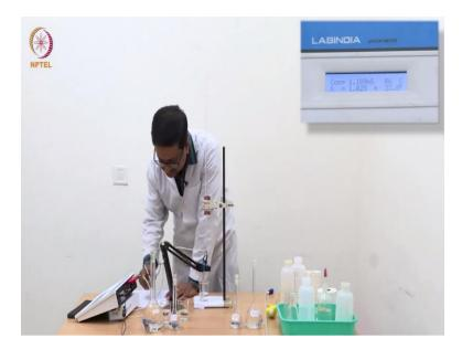
So, now I have added another 0.04 ml I have reached 0.08 ml and the conductance has reduced to 1.189. So, like that I am going to continue addition of 0.04 ml each time.
