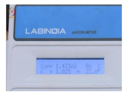
So, before we start the actual experiment I would like to explain a bit about this conductivity meter which you can see on your screen. The celcon standard we have here is calibrated to 1.025 and the conductance value that you are seeing here of 1.430 milli-siemens. This conductance is the conductance of a solution of 0.01 molar Kcl which I have prepared by accurate wing.
