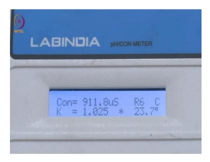
So, now I am adding this HCL to water which I have taken to emerge the electrode. You should notice in the reading that now the electrode is reading the concentration, reading the conductivity of the solution of HCL in water. I have to add completely as much as it goes and leaving the last drop here. So, now when I shake this solution well and homogenize this will then read the starting conductance of this particular titration.
