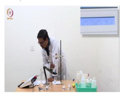
So, now our reading for 2.0 ml is 0.721 micro-siemens, sorry 721 micro-siemens or 0.721 milli-siemens. So, with this we will finish taking the readings of this experiment and we will use a standard graph paper to plot it, I will discuss how one can plot this numbers efficiently and get a very good end point through the theory lecture that will be followed after this
