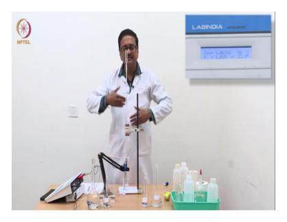
So, now I have reached a value of 0.2 ml and you see the reduced conductance is 1.087. So, like this again I will continue adding 0.04 ml and show you the reading after a few readings that I have already taken. So, now what you can see is that I have reached 0.4 ml of NaOH and the conductance has reduced in the level of micro-siemens, that is it is now giving you the reading in 937 which essentially means 0.937 milli-siemens.
