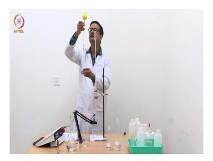
So, now to this water I will add N by 100 HCL solutions which is here which we prepared the other day the same HCL solution I am going to use for this analysis. So, this is approximately N by 100 HCL, I am going to add this N by 100 HCL 10 ml to this beaker. So, I will be getting out this N by 100 HCL using a 10 ml pipette and carefully making it up to the mark which is marked here as 10 ml. You can see there is a mark here which tells that this volume is 10 ml.
