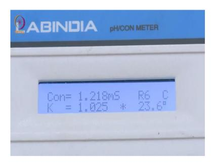
Now, I am going to use this 10 ml micro burette which I have filled with N by 10 NaOH and we will start adding small portions of N by 10 NaOH to this solution and mix the solution well, homogenize it and then take the reading of this changed conductance. So, now I am starting with addition of 0.04 ml of this NaOH solution. So, after adding 0.04 ml the conductance has changed to 1.218 milli-siemens.
