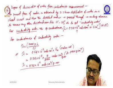
So, now let us try to see how can we estimate the degree of dissociation of water from conductance measurement, see for conductance measurement we need to get a very high-quality water which essentially should not be dissociated and should not be conducting electricity but that is practically impossible.
