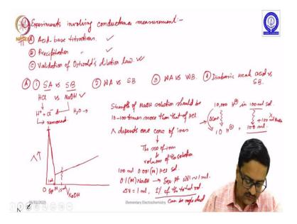
So, today we will start our discussion based on experiments involving conductivity measurement or conductance measurement. So, for this experiment what we need is the conductivity cell which we have drawn in the past and the cell should have a suitable electrode normally a platinum electrode of one square centimeter area kept at 1 centimeter apart and the cell constant is then what?
